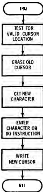
Fig. 2-19. Simplified flowchart of a typical Cursor control program.
