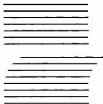
(C) Interrupted Scan more than one horizontal line—tears to the right.
