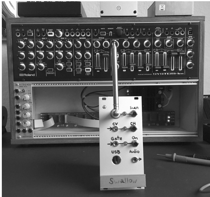
Figure 28.14 Early incarnation of the VC FM receiver controlled by Arduino for mapping stations to keyboard (made for Antonio de Luca).
