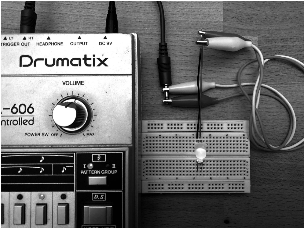
Figure 21.11 LED-controlled photoresistor with drum machine trigger input.
