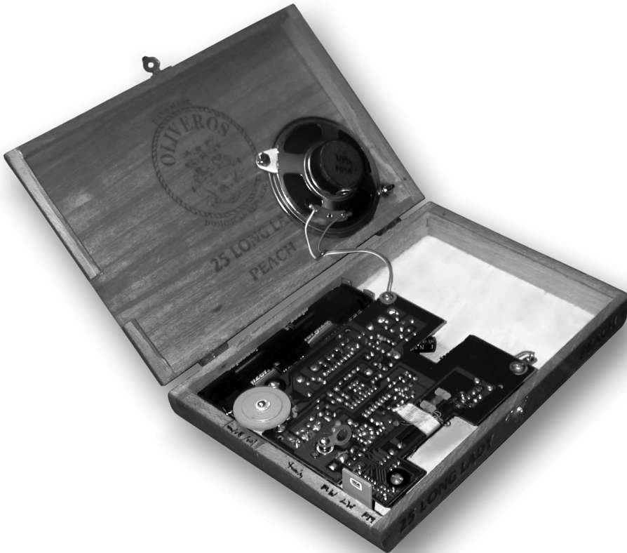
Figure 12.3 Nicolas Collins, Oliveros Radio-Cracklebox mounted inside a cigar box.
