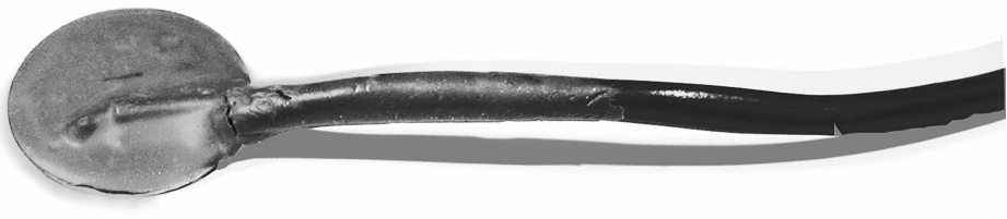
Figure 7.6 Contact mike encased in Plasti-Dip.
