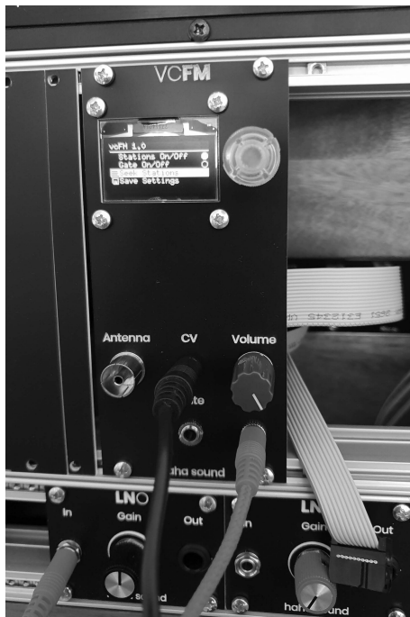
Figure 28.15 VC FM receiver controlled by Teensy 3.6 with graphical user interface and keyboard mapping.
