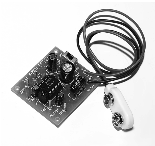
Figure 1.2 A low-power amplifier kit: assembled circuit board (left) and mounted in an Altoids tin (right).
