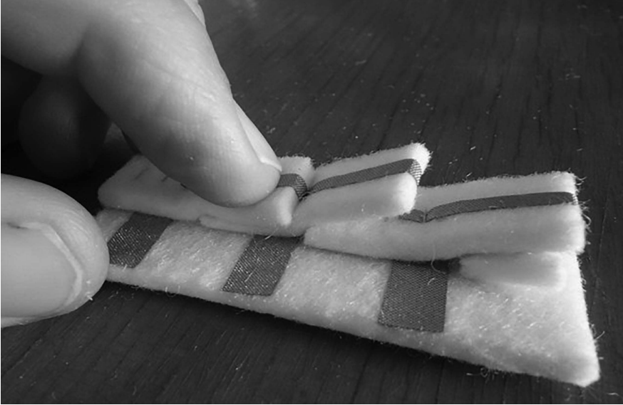
Figure 16.2 Hannah Perner-Wilson, stroke sensor that detects stroking direction.
