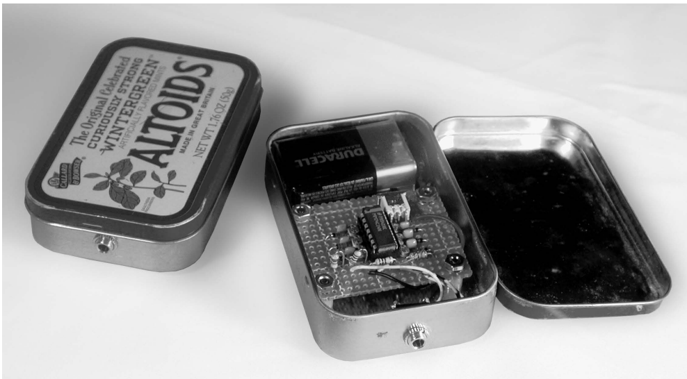
Figure 14.5 A boxed photoresistor-controlled hex oscillator.
