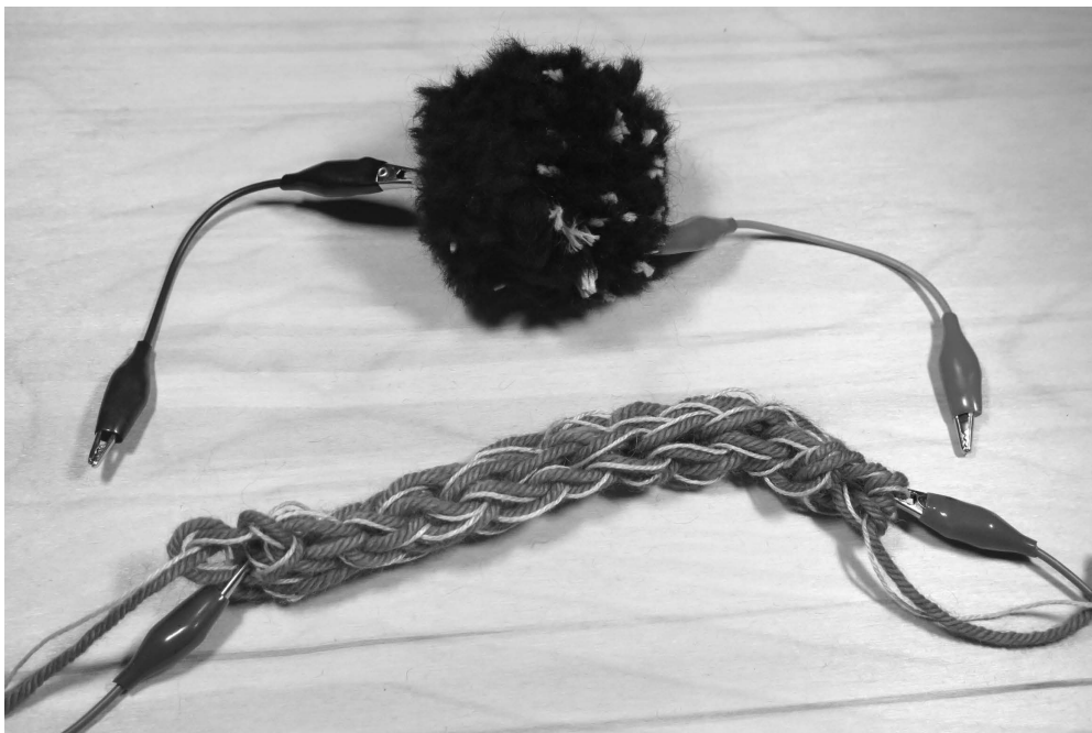
Figure 16.28 Completed pom-pom squeeze sensor and knitted stretch sensor.
