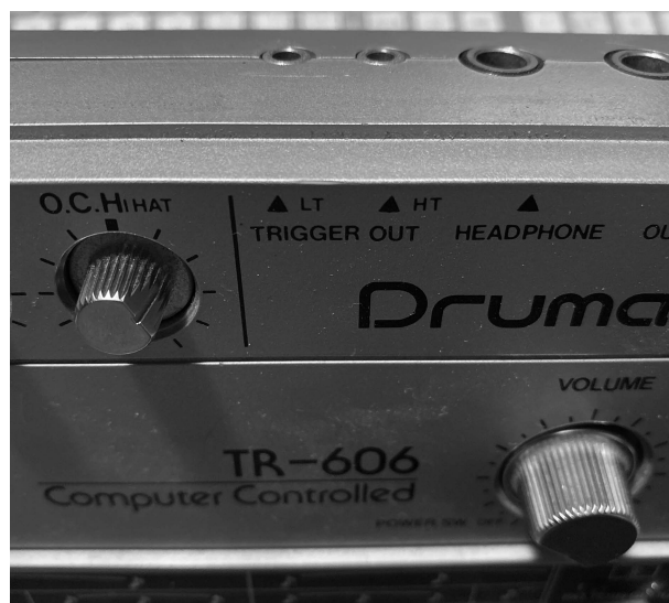
Figure 21.3 TR-606 trigger outputs (at top of image).
