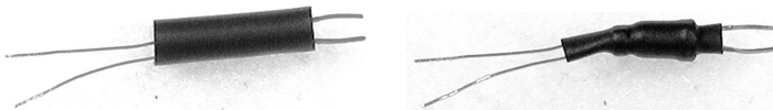
Figure 17.14 LED and photoresistor in heat-shrink tubing, before shrinking (left) and after shrinking (right).
