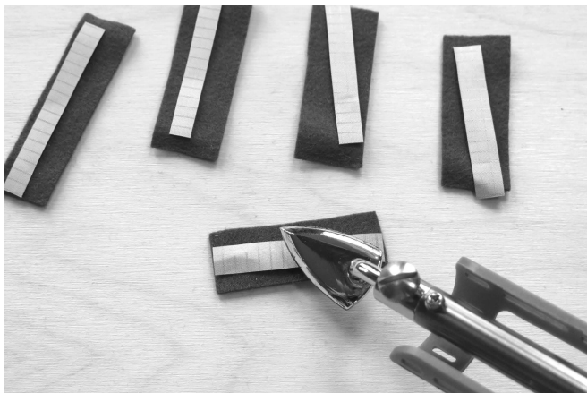
Figure 16.32 Ironing down the conductive fabric onto the felt.
