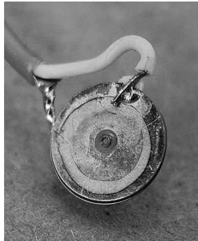
Figure 7.14 Element from ultrasonic transducer wired to shielded cable for use as contact mike.
