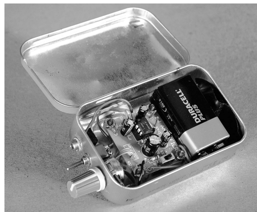
Figure 1.2 A low-power amplifier kit: assembled circuit board (left) and mounted in an Altoids tin (right).
