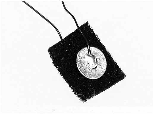
Figure 13.16 Pressure sensor made from anti-static foam between two coins.
