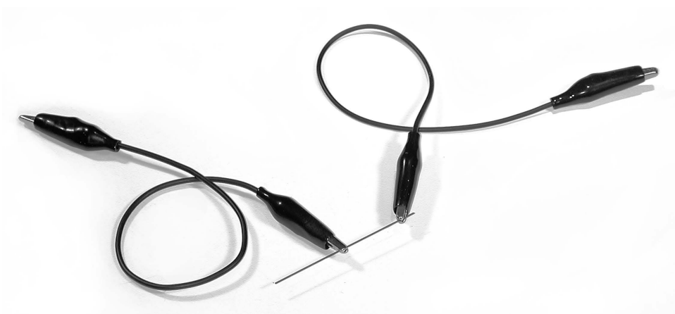
Figure 13.17 A pencil-lead resistor.
