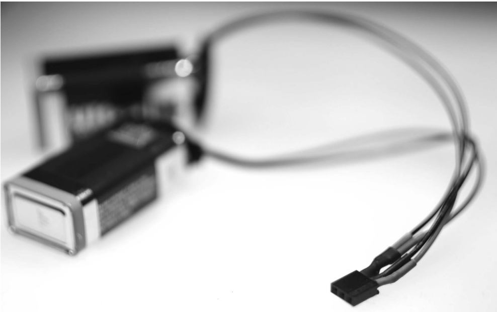
Figure 31.5 Powering the Confetti Neuron from two 9-volt batteries.
