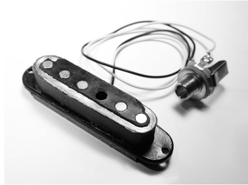
Figure 6.7 A guitar pickup with case broken away to reveal internal coil.
