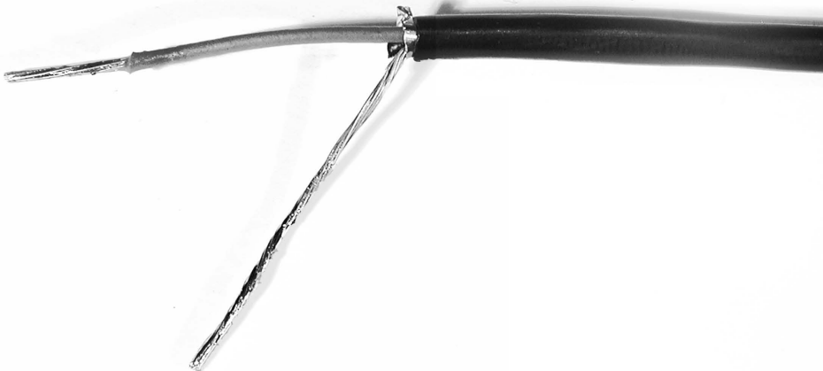
Figure 7.2 Shielded cable prepared for soldering.
