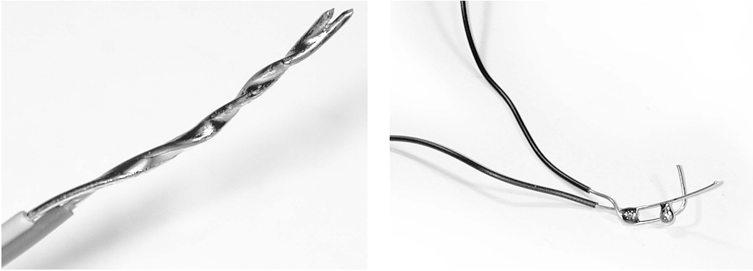
Figure 5.5 A happy solder joint (left) and a sad solder joint (right).
