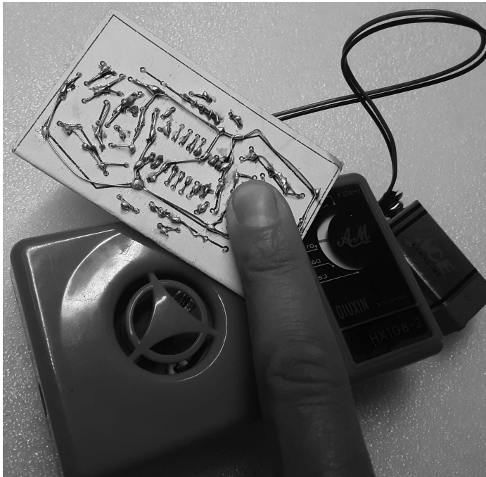
Figure 26.6 Jamming an AM radio. Gentle fingering on the nodes will further mangle the sound.
