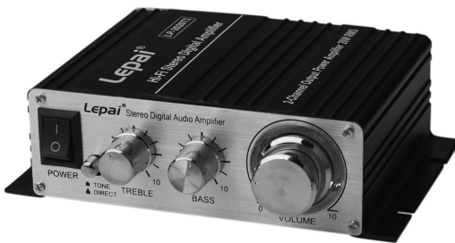
Figure 1.3 Typical low-power class D stereo amplifier.
