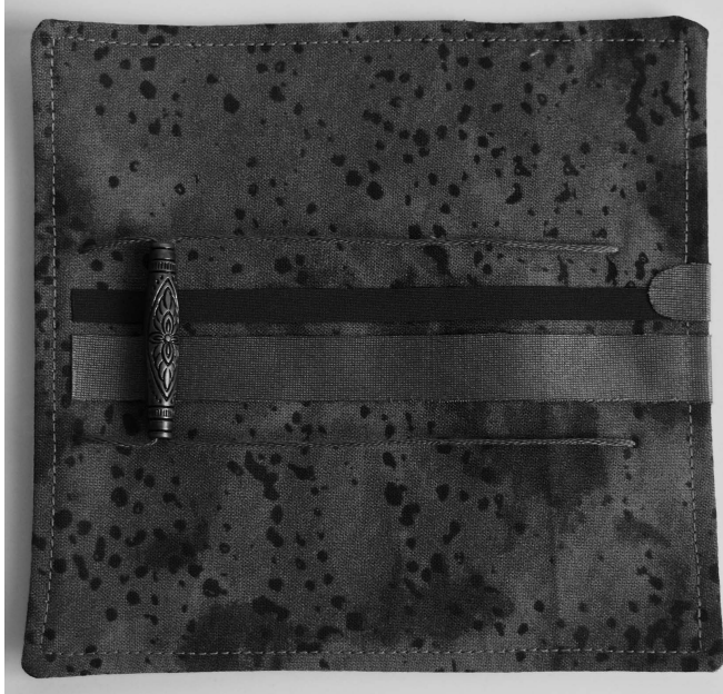
Figure 16.4 Liza Stark, linear potentiometer.
