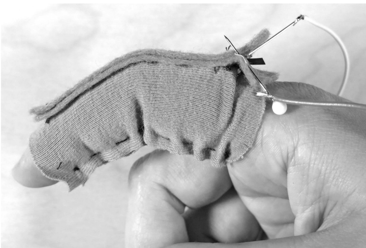
Figure 16.43 Sewing the sleeve's seam; finished sleeve with sensor on finger.
