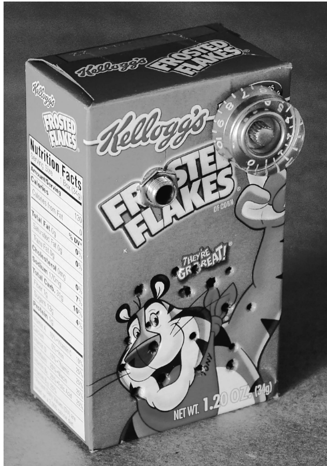
Figure 24.5 Mini-amplifier built from LM386.
