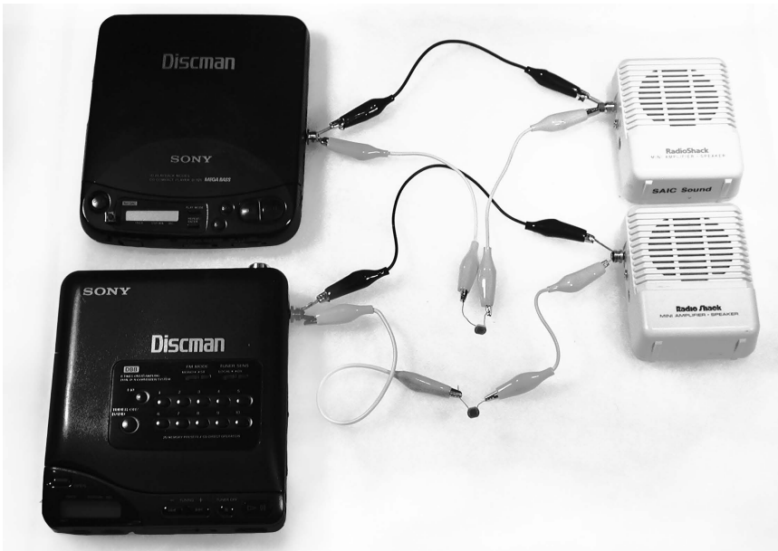
Figure 17.5 Patchable optical panner/mixer.
