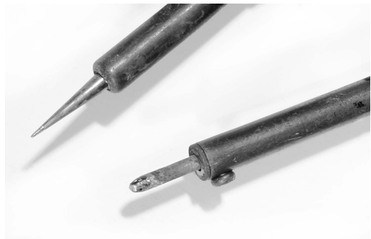
Figure 5.2 A happy soldering iron (top) and a sad soldering iron (bottom).
