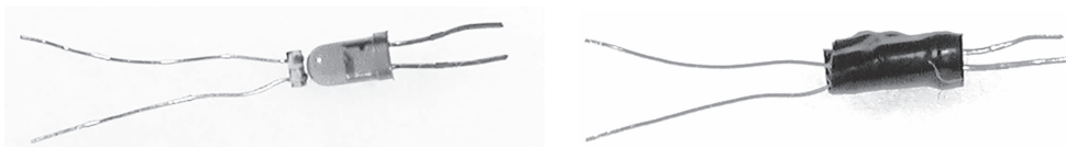
Figure 17.10 LED and photoresistor kissing (left) and bundled in electrical tape (right).
