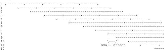
This method of choosing offsets for subblocks can result in an occasional small offset (as shown above) between one pass and the next, particularly when G is large compared to J. For example:
