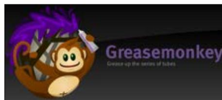
Greasemonkey is a Firefox plugin that allows users to install scripts that make on the fly changes to web page content before or after the page is loaded. Greasemonkey can be used for customizing a web page appearance, web functions, debugging, combining data from other pages, as well as other purposes. Greasemonkey is required to make other tools, such as Cookie Injector, function properly.
