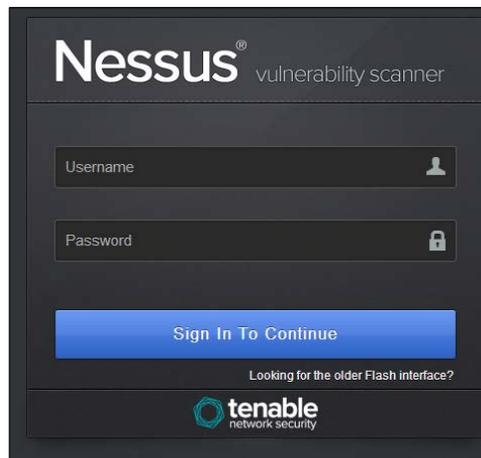
To start a scan, click on the **Scan** tab on the top ribbon and select **New Scan**. You will be then prompted to enter details of the target. You will also be asked to select what template you would like to use. Nessus has a few built-in templates. In this example, we are choosing external network scan.
