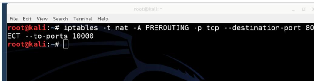
A terminal window titled 'root@kali: ~' with a menu bar (File, Edit, View, Search, Terminal, Help). The terminal shows the command 'iptables -t nat -A PREROUTING -p tcp --destination-port 80' and its output 'ECT --to-ports 10000'. The prompt returns to 'root@kali:~#'.
