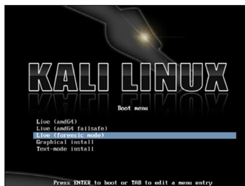
Using Kali in **Forensic mode** helps you achieve your number one golden rule of not modifying the original filesystem. The internal hard drive is not touched and there is no automount of internal disks. Swap partitions and any other memory or caching partitions are also not used in any way.
