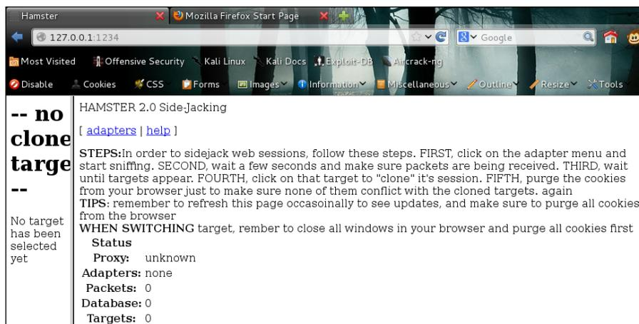
Traffic must travel through Hamster for it to do its job. You can select which adapter to use by clicking the adapters link. For my example, I'm going to sniff **eth0**.
