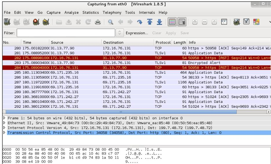
Wireshark captures a lot of details, so it is important to filter for specific things, such as parameters for unsecured cookies like `http.cookie`. For example, Gmail by default is encrypted; however, you can turn off `https` and seek out the `GX` parameter contained in a `http.cookie` to identify unsecured Gmail cookies. The following screenshot shows capturing the cookie from logging into a Wordpress blog:
