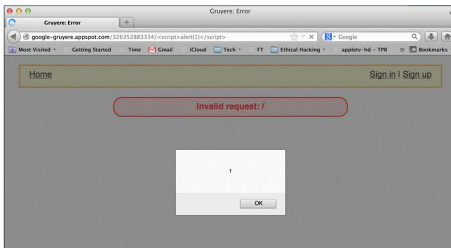
The example shows our target web application server issue a popup proving that this site is vulnerable to an attack. We can use ZAP to replay the attack, try other attacks, or test similar XSS methods.
