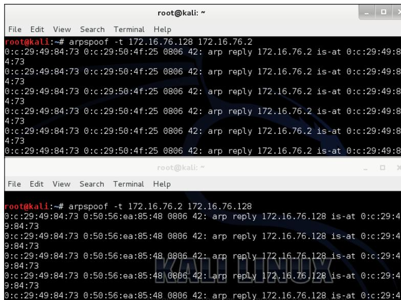
If you enter the commands correctly, you should see that traffic is being replayed through the attacking system. Traffic is not going to and from the victim, so the victim would not see traffic going out of the network at this point. To complete the attack, you need to enable IP forward so traffic will continue to flow from the default gateway to the victim and vice versa, while the attacker is watching traffic between the victim and default gateway.
