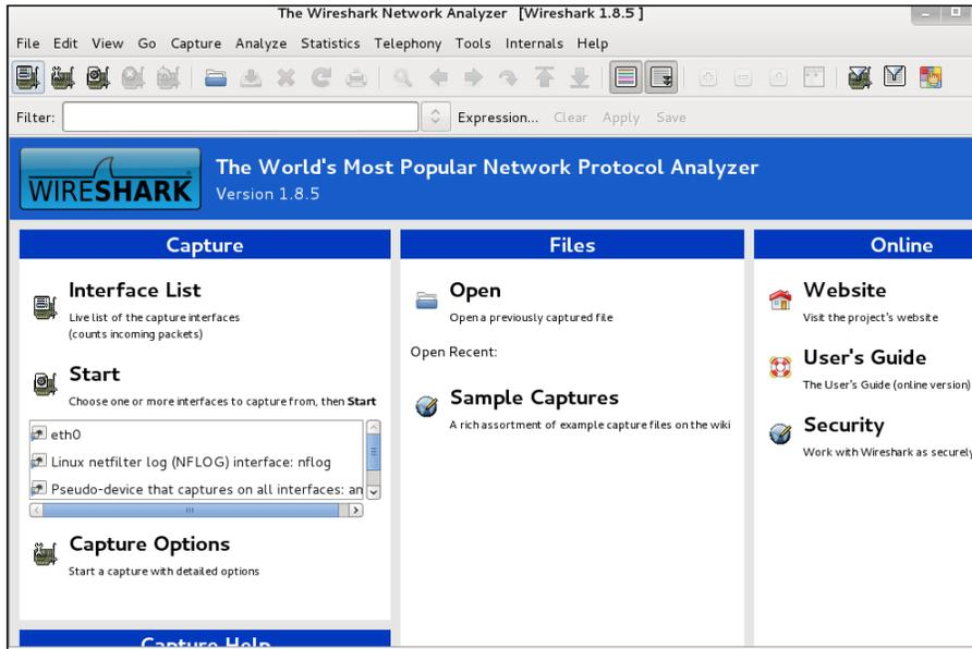
To start capturing traffic, select the **Capture** tab and **Interfaces**. You will see the available interfaces to capture. In my example, I'm going to select **eth0** by clicking on the checkbox next to **eth0** and selecting **Start**.
