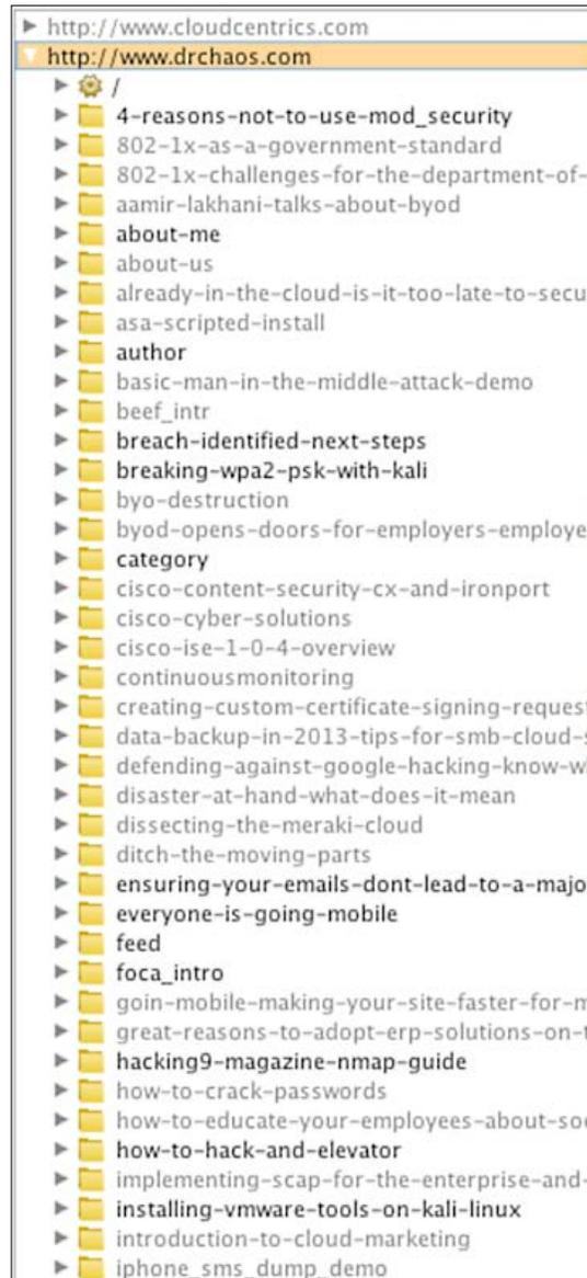
Burp shows all pages and links that the **Spider** process has captured. In addition, it will capture the root directory, web page styles, sub-folders, and Java scripts. The next example shows multiple, captured sub-folders on the site [www.Drchaos.com](http://www.Drchaos.com).
