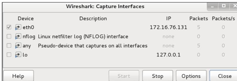
Wireshark will capture all traffic seen on the wire. Traffic can be filtered by typing specific items in the filter space or by adjusting the organization of data via the top tables, such as protocol or destinations.
