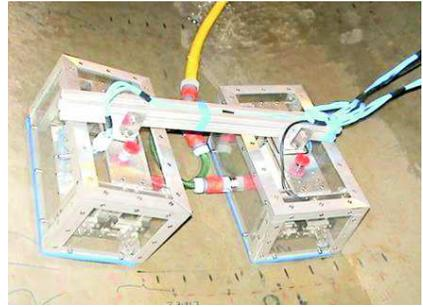
**Fig. 8.** Acoustic sensor systems for crack detection
