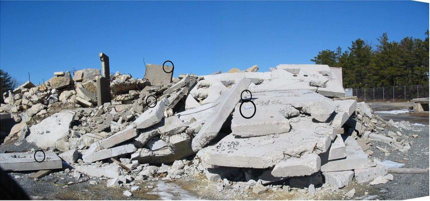
**Fig. 1.** Wide angle view of sensors placed on rubble. Most of the sensors are behind outcroppings and hence are not visible. The circles show the locations of a few of the sensors.
