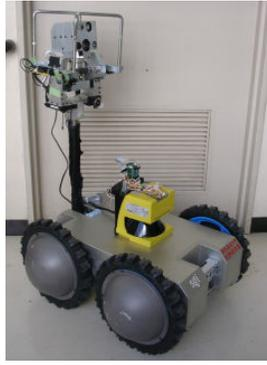
**Fig. 4.** A four-wheeled rescue robot FUMA with LRF. FUMA has five cameras and one on the top of the arm is used for the experiment. The yellow box on the body of the FUMA is the laser rangefinder, RS4-4 which is used as a positioning sensor.
