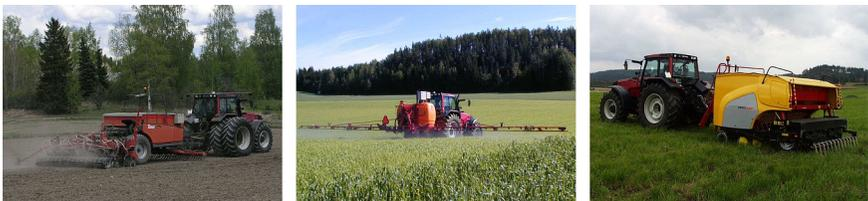
**Fig. 1.** Pneumatic drill, sprayer and no-tillage drill
