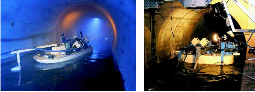
Fig. 1. Spy prototype and test of the swimming inspection system in a real sewer
