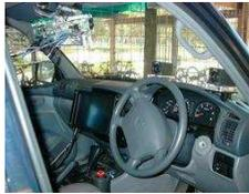
**Fig. 5.** Inside the ANU/NICTA intelligent vehicle. Cameras to monitor the road scene and find obstacles appear in place of the rear-vision mirror.
