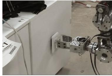
**Fig. 15.** Insertion with compliance motion
