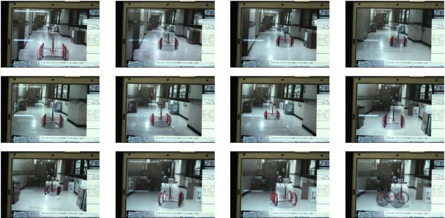
**Fig. 8.** Example of FOV evaluated image teleoperation. The snapshots of the experiment are represented from the left to the right and from the upper row to the bottom one as time goes by.
