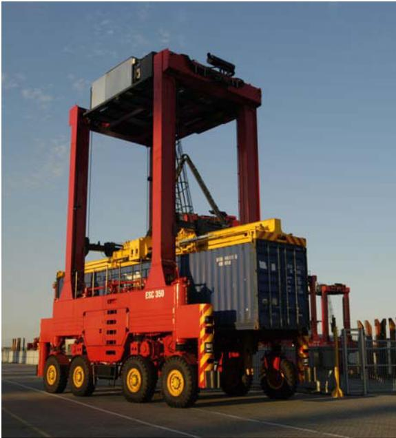
ment System and then transferred to the straddle carrier's Vehicle Management System. The execution system then tracks execution of these actions relative to the planned path by comparison with navigation system output. A number of methods are employed for evaluating path and control execution integrity during motion.
