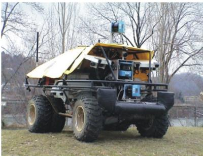
Fig. 1. The PerceptOR off-road mobile robot. The experiments were performed with this and similar vehicles.
