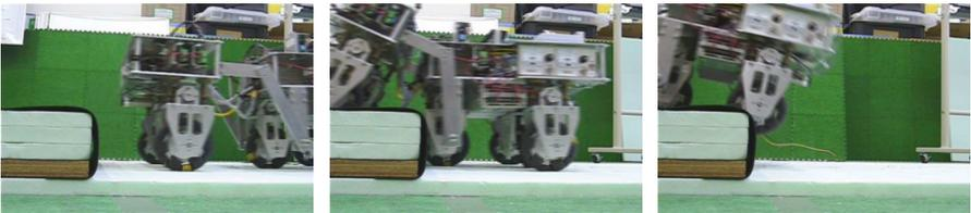
**Fig. 9.** Passing over the 152[mm] height step
