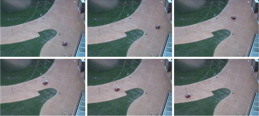
**Fig. 7.** Six snapshots of a guided navigation experiment. The Mica Motes are located as shown in Fig. 6. The optimal node sequence is 2, 3, 4, 9, 13, 16, 19. Because the viewing angle is not directly from above and there is some distortion in the net, the robot does not line up exactly with the node locations.
