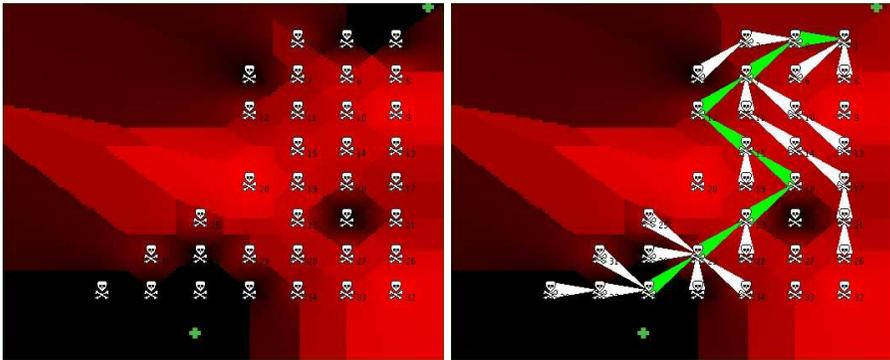
**Fig. 5.** (Left) Potential field danger map computed by sensors in response to the simulated presence of a chemical agent. (Right) Safest path computed for a trapped first responder by the sensor field.
