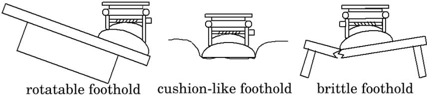
Fig. 14. three detectable footholds with sole sensors
