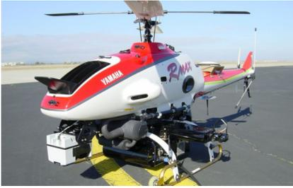
**Fig. 1.** The NASA/ARP helicopter equipped with a range measurement device from SICK.
