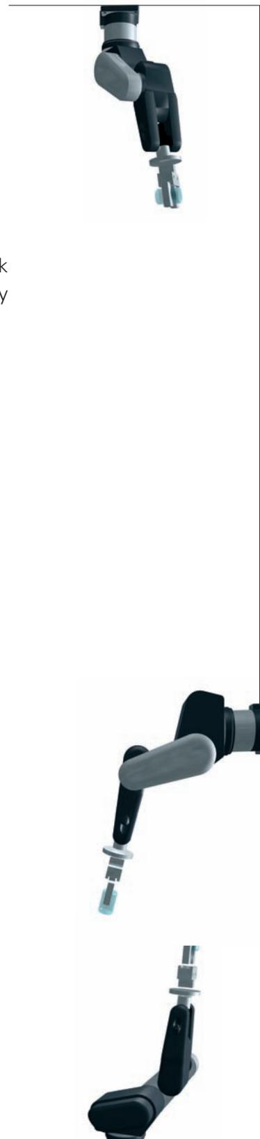
*Various mounting options for 5-axis robots – to ceiling, wall, and floor*
