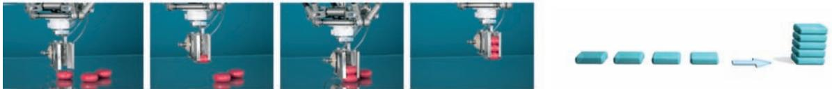
Pick operation of stack gripper
