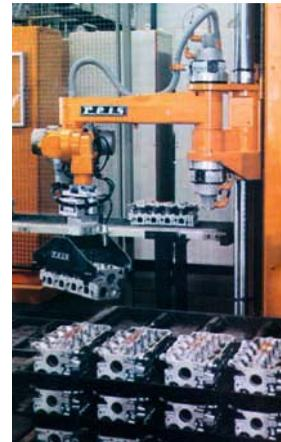
*ROBOT 625 handling motor blocks (source: Fraunhofer IPA)*
