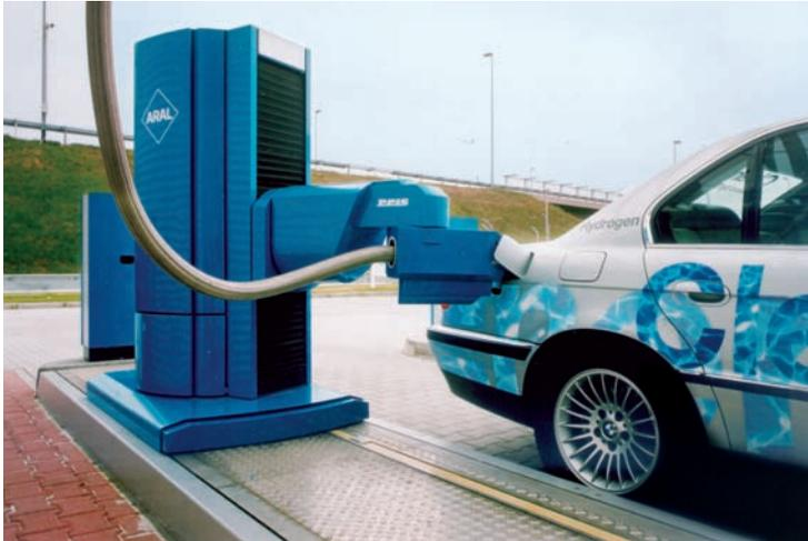
A possible trend in robot and automation component technology can be seen in the pictures of service robots venturing from factory halls into “unstructured” environments. During refueling, for example, a robot has to deal with a technical object, i. e. the car, but situations and fabricates vary. Robot fueling technology is being tested worldwide for filling up liquid hydrogen.
