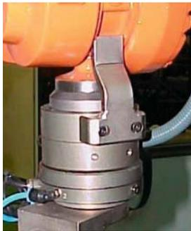
*Rotary distributor with torque reactor strut*
