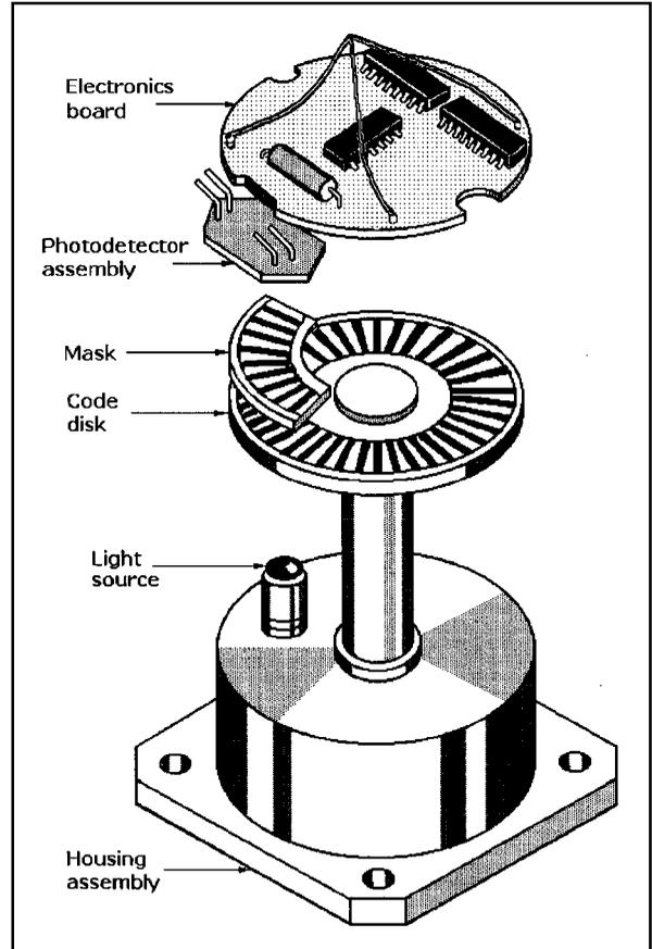
**Figure 1-35** Exploded view of an incremental optical rotary encoder showing the stationary mask between the code wheel and the photodetector assembly.
