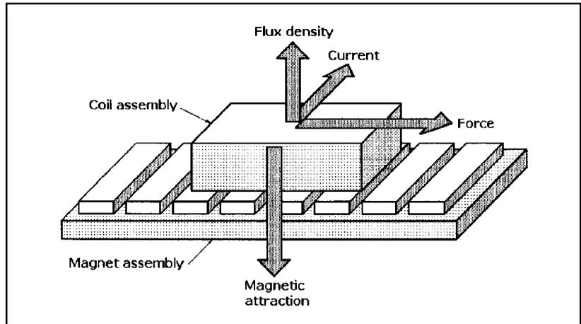
**Figure 1-27** Operating principles of a linear servomotor.
