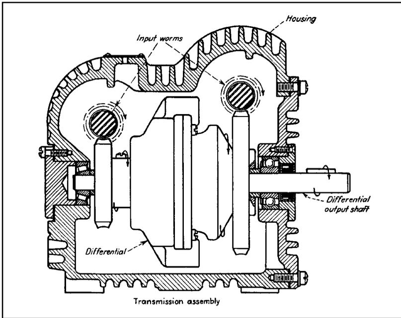
**Figure 2-20** A variable-speed transmission consists of two sets of worm gears feeding a differential mechanism. The output shaft speed depends on the difference in rpm between the two input worms. When the worm speeds are equal, output is zero. Each worm shaft carries a cone-shaped pulley. These pulley are mounted so that their tapers are in opposite directions. Shifting the position of the drive belt on these pulleys has a compound effect on their output speed.
