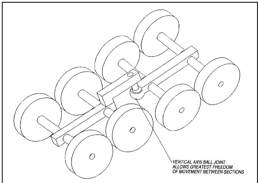
Figure 4-31 Two part, eight wheeled, vertical ball joint
