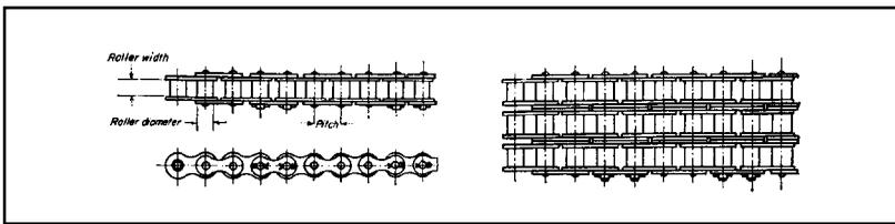
**Figure 2-10a** Standard roller chain—for power transmission and conveying.
