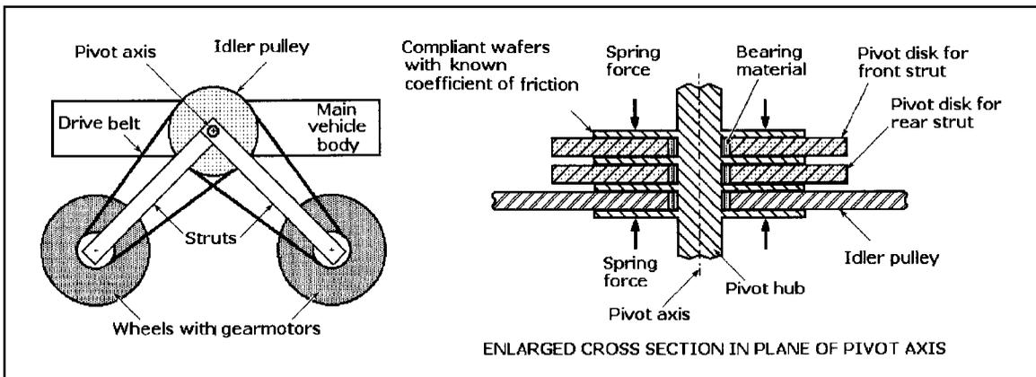
**Figure 4-14** Each wheel is driven by a dedicated gearmotor and is coupled to the idler pulley. The pivot assembly imposes a constant frictional torque  $T$ , so that it is possible to (a) turn both wheels in unison while both struts remain locked, (b) pivot one strut, or (c) pivot both struts in opposite directions by energizing the gearmotors to apply various combinations of torques  $T/2$  or  $T$ .
