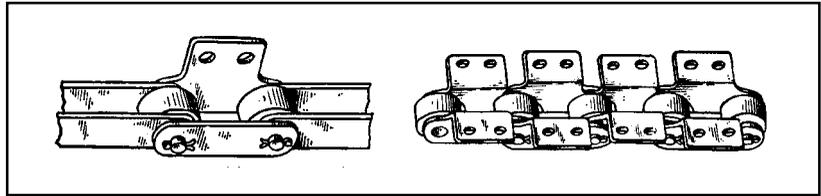
Figure 2-11 Bent lug roller chain used for rack and pinion linear actuator.
