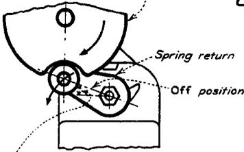
Small operating angle assures drift of machine returns lever to off position for next angle
