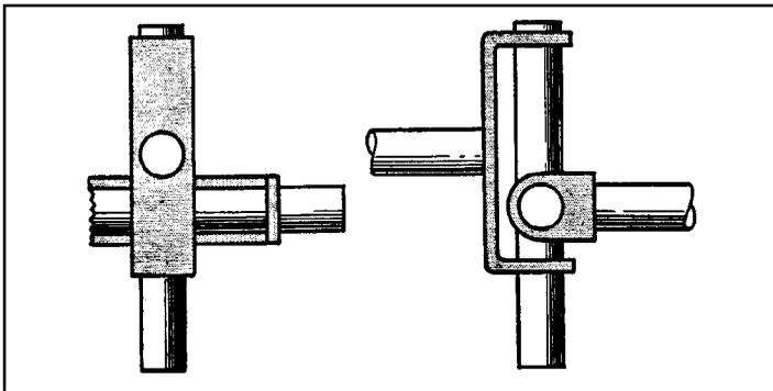
**Figure 3-32** This crossed-axis yoke coupling is a variation of the mechanism shown in Fig. 2. Each shaft has a yoke connected so that it can slide along the arms of a rigid cross member. Transmission is at a constant velocity, but the shafts must remain parallel, although the offset can vary. There is no axial freedom. The central cross member describes a circle and is thus subjected to centrifugal loads.
