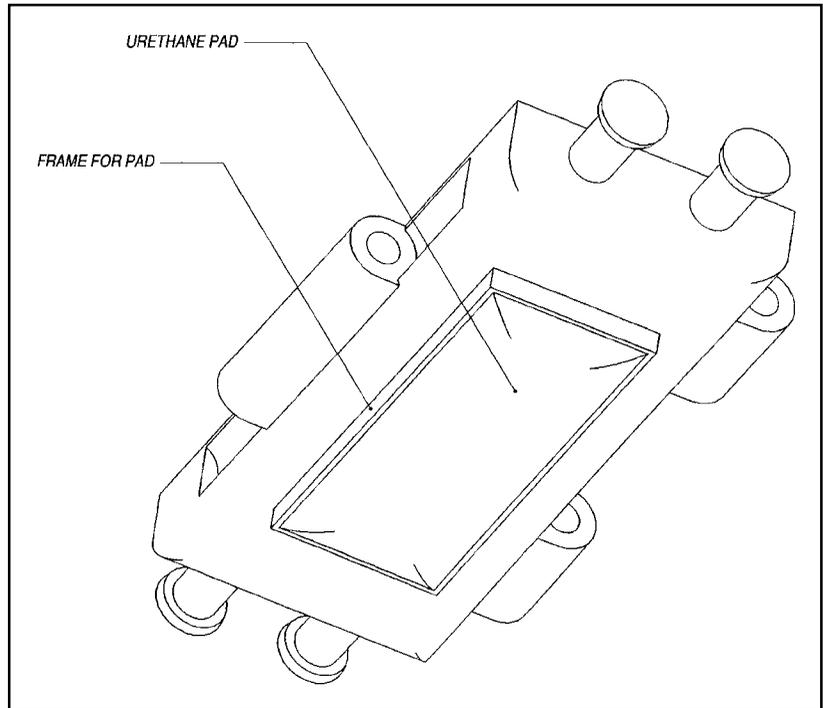
Figure 5-3 Urethane pads for hard surface roads
