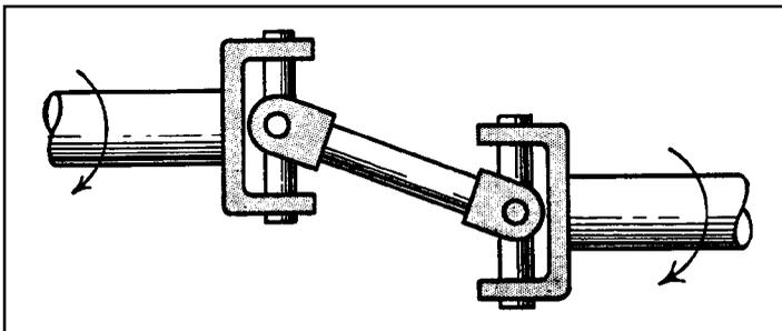
**Figure 3-31** This coupling consists of two universal joints and a short shaft. Velocity transmission is constant between the input and output shafts if the shafts remain parallel and if the end yokes are arranged symmetrically. The velocity of the central shaft fluctuates during rotation, but high speed and wide angles can cause vibration. The shaft offset can be varied, but axial freedom requires that one shaft be spline mounted.
