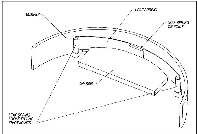
Figure 11-16 Horizontal loose footed leaf spring
