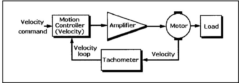
Figure 1-4 Block diagram of a velocity-control system.
