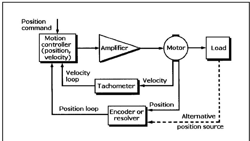
Figure 1-5 Block diagram of a position-control system.
