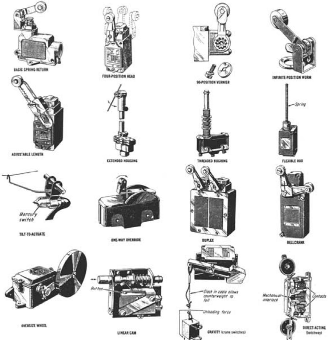
Figure 11-5a Mechanical, Geared, and Cam Limit Switches
