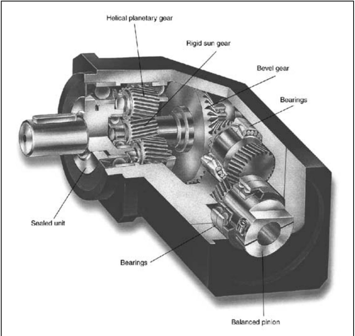
**Figure 2-28** This right-angle gearhead is designed for high-performance servo applications. It includes helical planetary output gears, a rigid sun gear, spiral bevel gears, and a balanced input pinion. *Courtesy of Bayside Controls Inc.*
