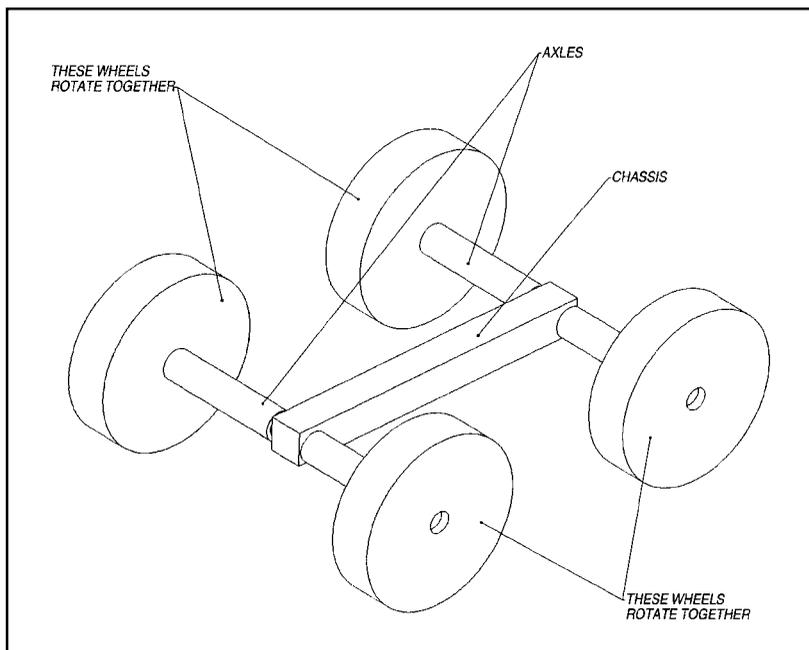
**Figure 4-10** All four fixed, skid steered
