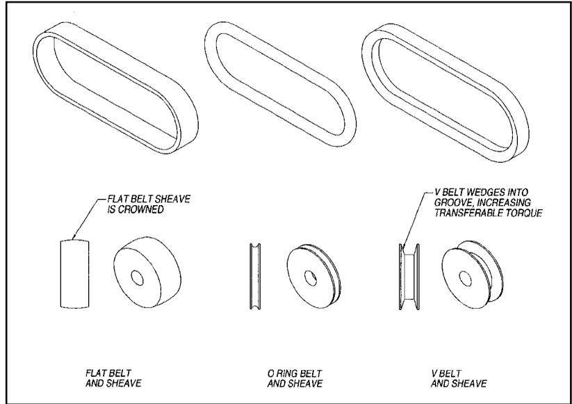
Figure 2-1 Flat, O-ring, and V-belt profiles and pulleys
