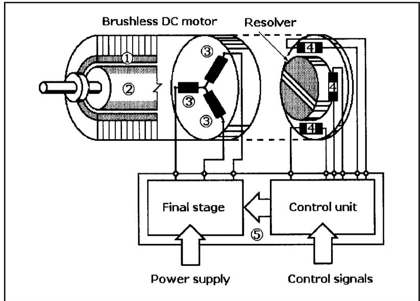
**Figure 1-26** A resolver as a rotor position indicator: stationary motor winding (1), permanent-magnet motor rotor (2), three-phase electronically commutated field (3), three magnetic sensors (4), and the electronic circuit board (5).
