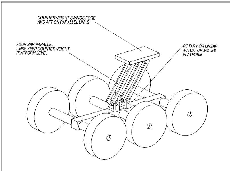
Figure 4-2 Shifting the cg on a swinging arm
