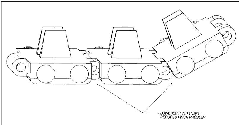
**Figure 5-2** Effective hinge location of all-steel track
