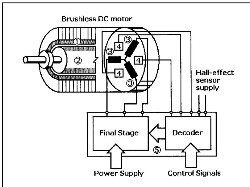
**Figure 1-25** A magnetic sensor as a rotor position indicator: stationary brushless motor winding (1), permanent-magnet motor rotor (2), three-phase electronically commutated field (3), three magnetic sensors (4), and the electronic circuit board (5).
