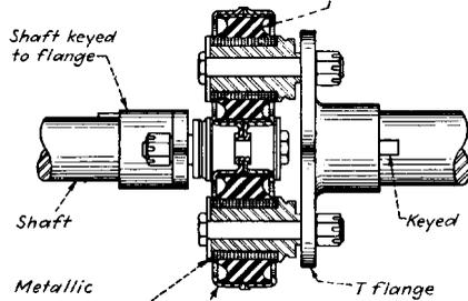
Outer fabric ring impregnated with neoprene, provides support for center section
