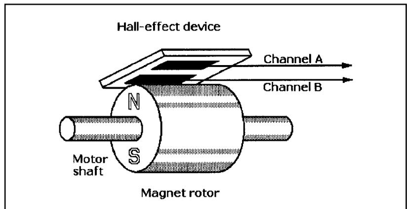
Figure 1-39 Basic parts of a magnetic encoder.
