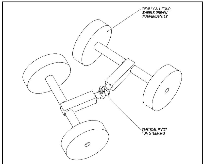
**Figure 4-18** Two-sections connected through vertical axis joint
