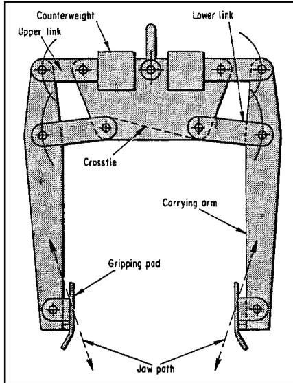
Figure 10-24 Passive parallel jaw using cross tie
