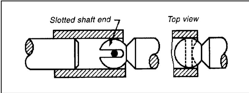
**Figure 3-23** A pinned-sleeve shaft-coupling is fastened to one shaft that engages the forked, spherical end on the other shaft to provide a joint which also allows for axial shaft movement. In this example, however, the angle between shafts must be small. Also, the joint is only suitable for low torques.
