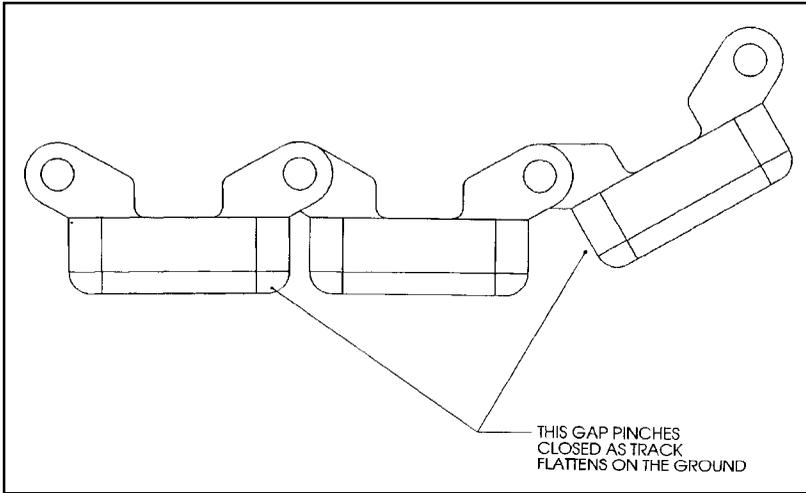
**Figure 5-1** Basic steel link layout showing pinch point
