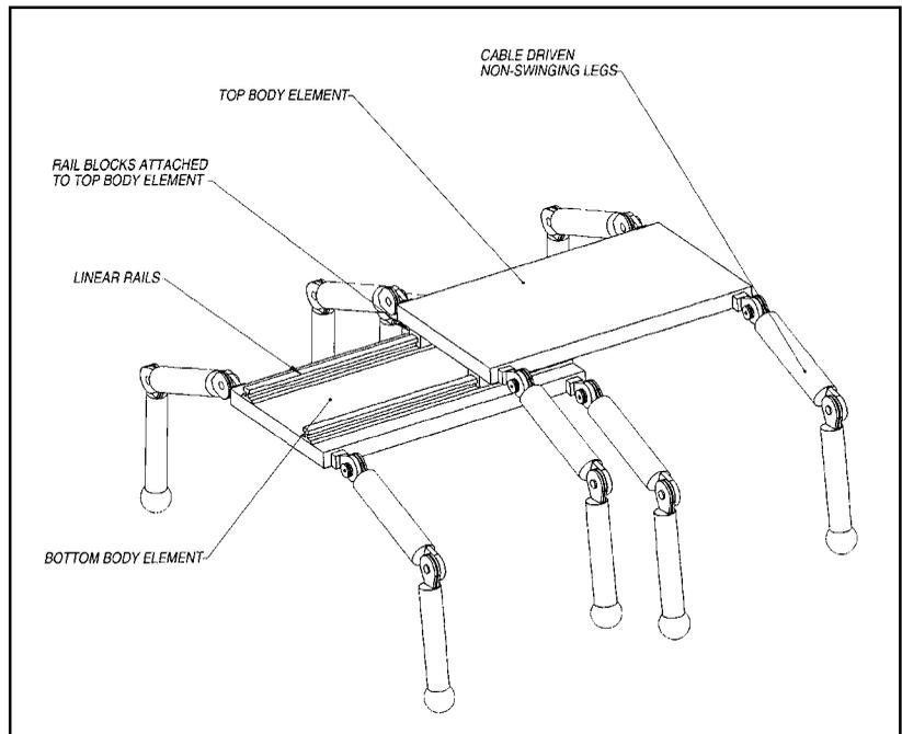
**Figure 7-13** Eight-leg frame walker with two-DOF legs
