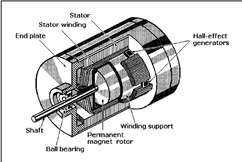
Figure 1-22 Cutaway view of a brushless DC motor.
