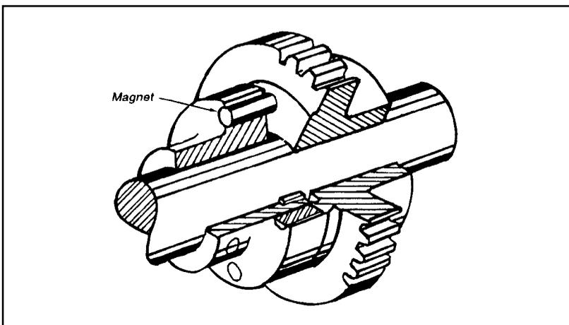
**Figure 3-44** Permanent magnets transmit torque in accordance with their numbers and size around the circumference of the clutch plate. Control of the drive in place is limited to removing magnets to reduce the drive's torque capacity.
