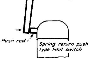
Switch operation      No switch operation
