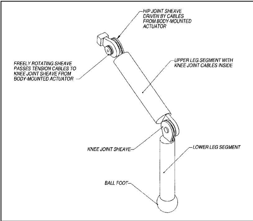
Figure 7-5 Two-DOF leg using cable driven actuators
