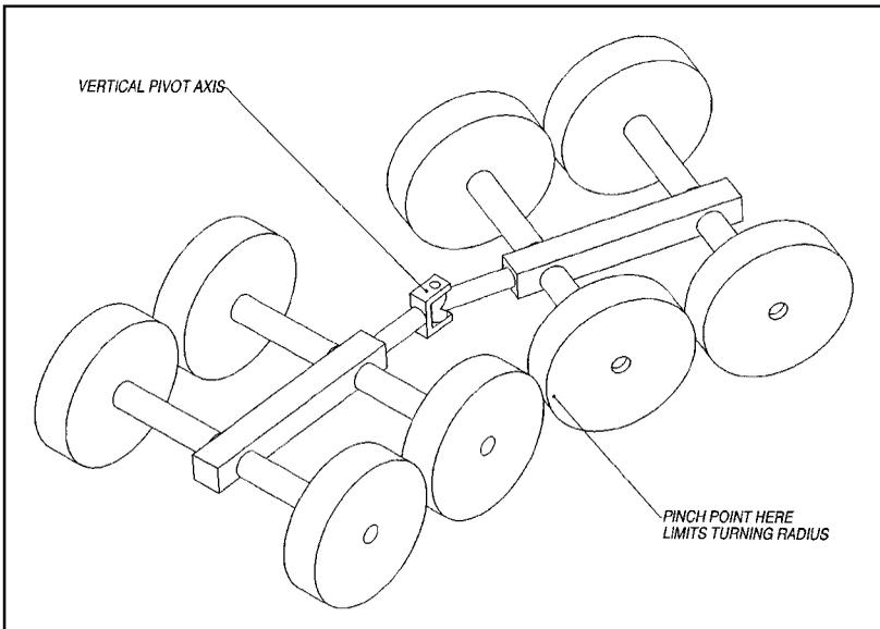
**Figure 4-29** Two part, eight wheeled, vertical center pivot
