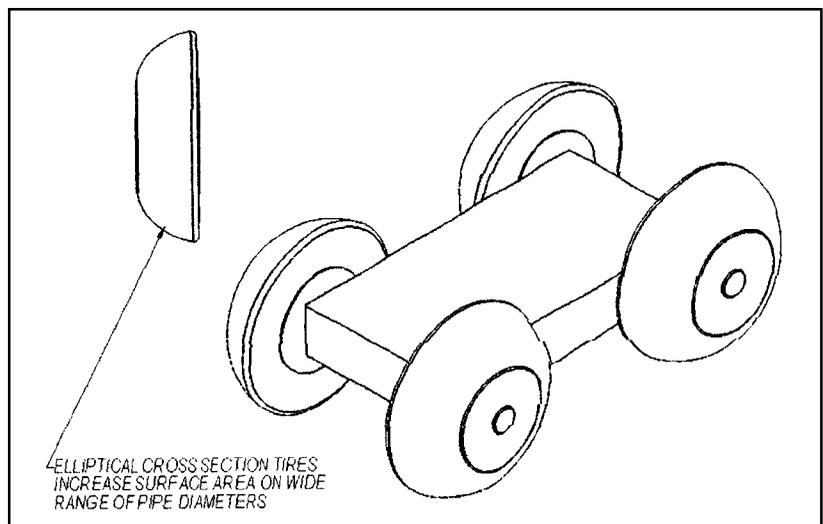
Figure 8-1 Four-wheeled horizontal pipe crawler
