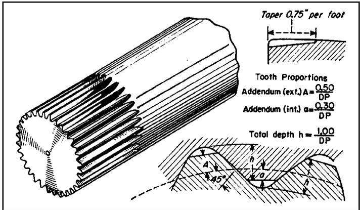
**Figure 3-36** Straight-Sided splines have been widely used in the automotive field. Such splines are often used for sliding members. The sharp corner at the root limits the torque capacity to pressures of approximately 1,000 psi on the spline projected area. For different applications, tooth height is altered, as shown in the table above.
