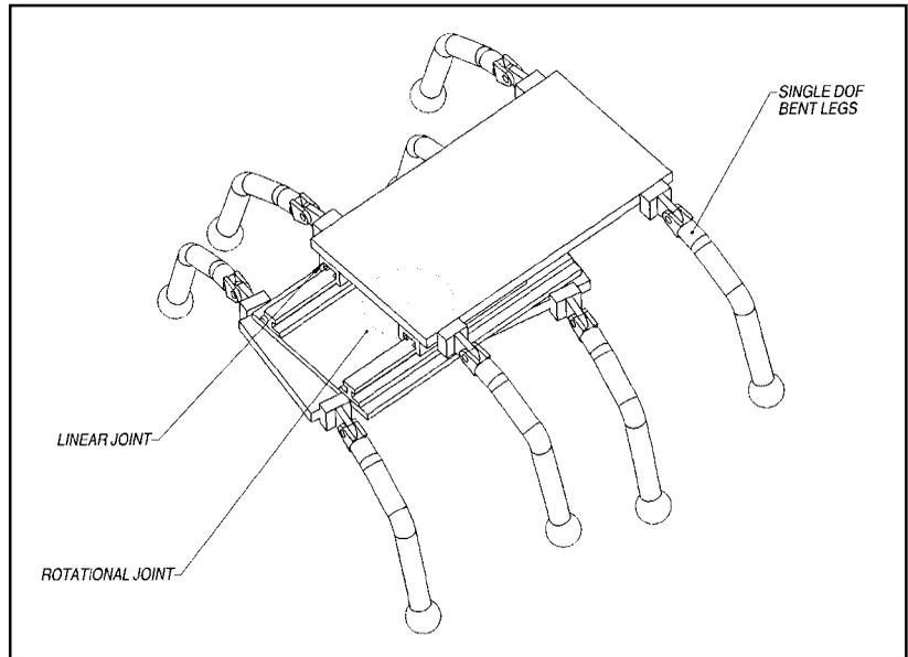
**Figure 7-12** Traversing/rotating frame eight-leg walker with single-DOF legs
