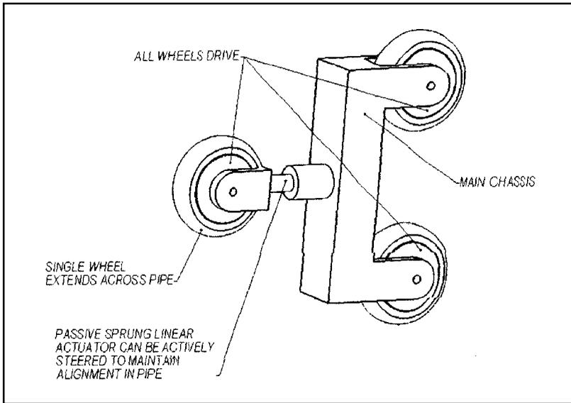
Figure 8-3 Basic three-wheeled
