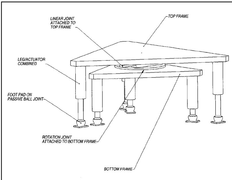
**Figure 7-14** Six-legged tripod-frame walker with single-DOF legs
