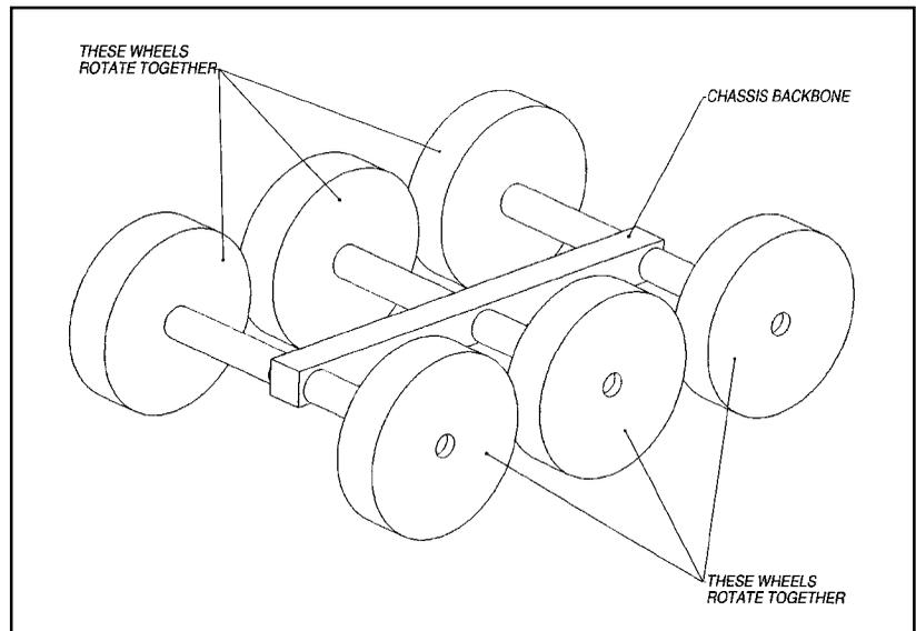
**Figure 4-21** Six wheels, all fixed, skid steer
