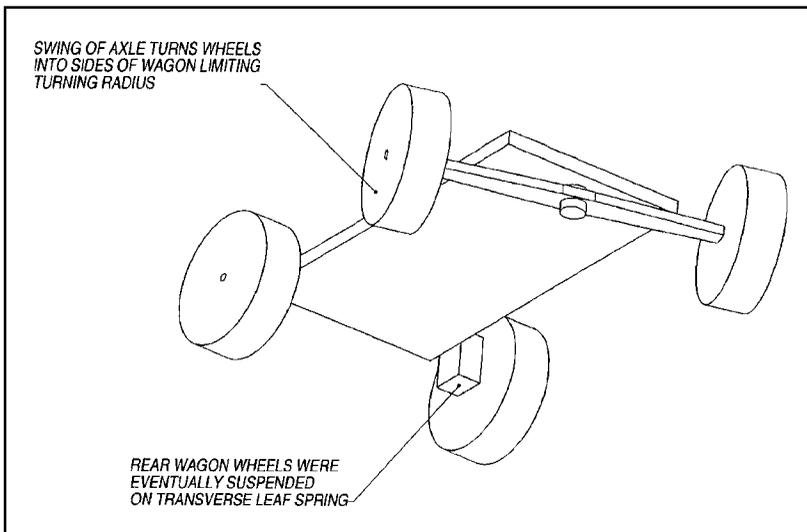
Figure 6-1 Pivot mounted front wheels
