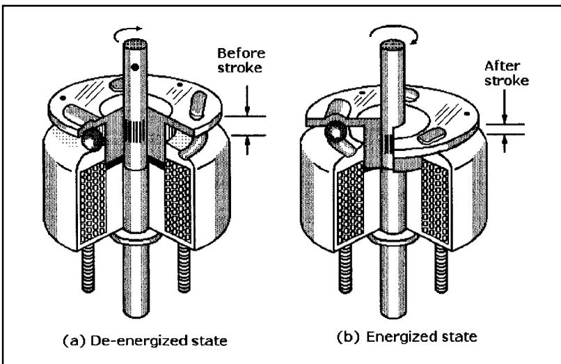
**Figure 1-53** Cutaway views of a rotary solenoid de-energized (a) and energized (b). When energized, the solenoid armature pulls in, causing the three ball bearings to roll into the deeper ends of the lateral slots on the faceplate, translating linear to rotary motion.
