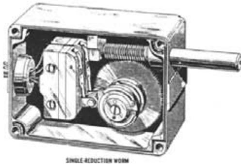
**Rotary-Cam Limit Switches**
