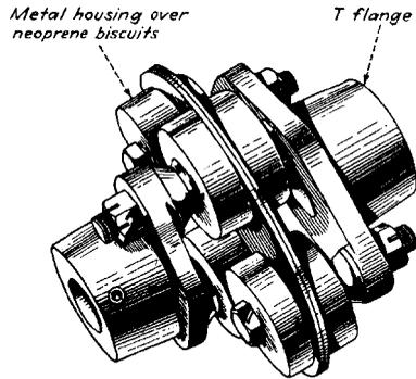
Neoprene center designed for uniform stress, linear deflection and absorption of vibration
