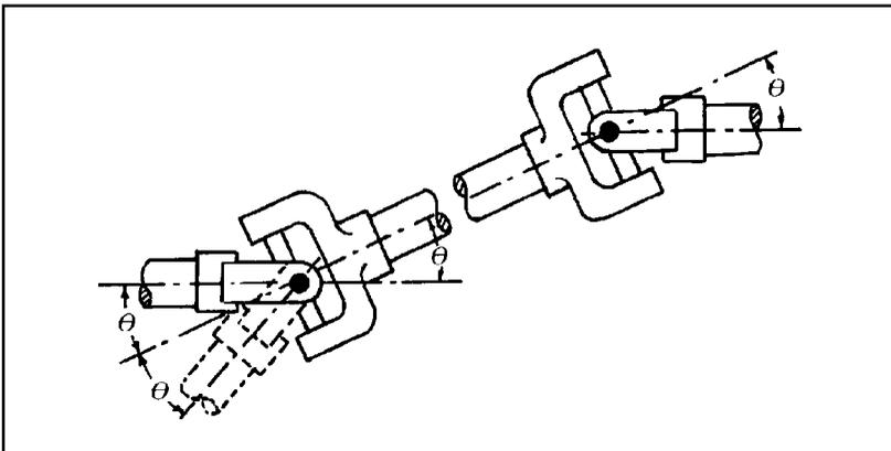
**Figure 3-24** A constant-velocity joint is made by coupling two Hooke's joints. They must have equal input and output angles to work correctly. Also, the forks must be assembled so that they will always be in the same plane. The shaft-alignment angle can be double that for a single joint.
