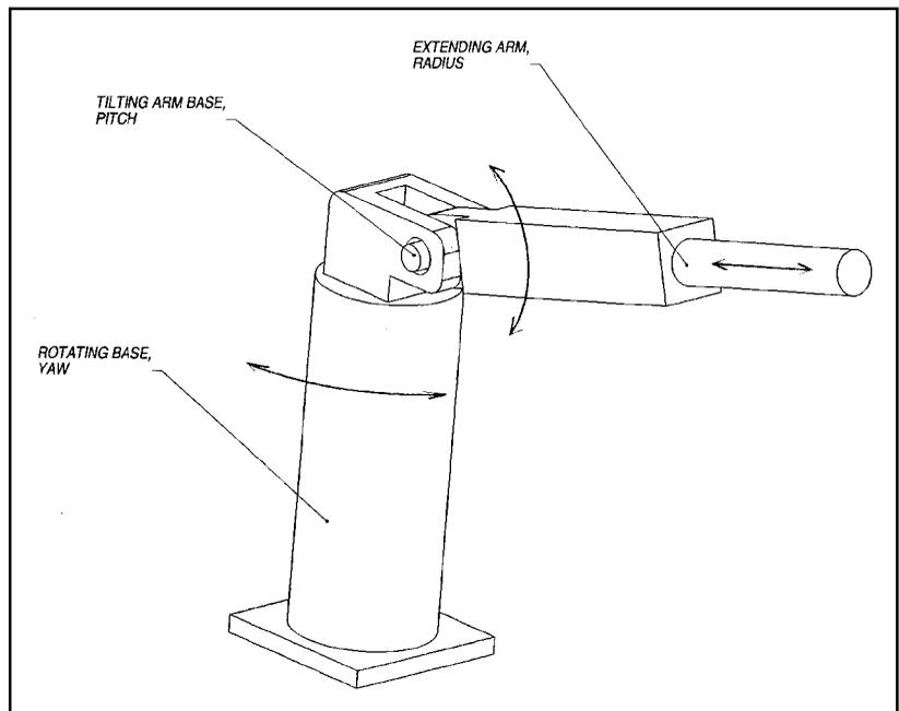
Figure 10-9 High shoulder polar coordinate manipulator with offset joint at elbow
