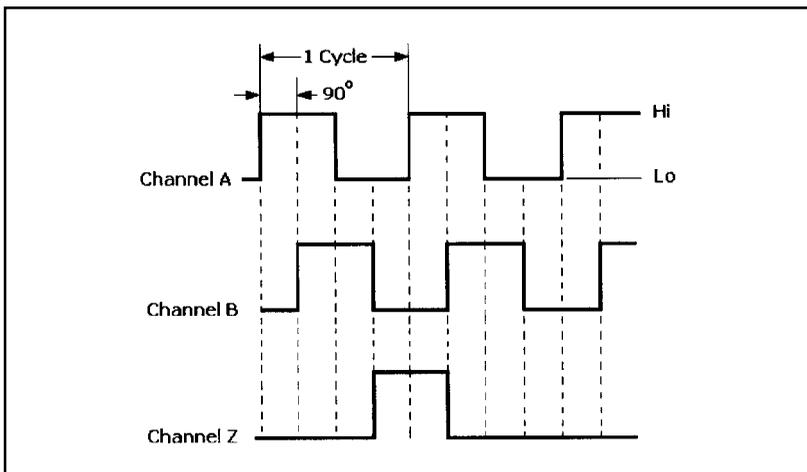
**Figure 1-36** Channels A and B provide bidirectional position sensing. If channel A leads channel B, the direction is clockwise; if channel B leads channel A, the direction is counterclockwise. Channel Z provides a zero reference for determining the number of disk rotations.
