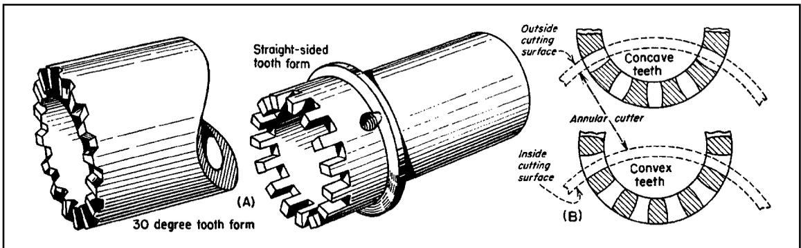
**Figure 3-43** Curvic Coupling teeth are machined by a face-mill cutter. When hardened parts are used that require accurate positioning, the teeth can be ground. (A) This process produces teeth with uniform depth. They can be cut at any pressure angle, although 30° is most common. (B) Due to the cutting action, the shape of the teeth will be concave (hour-glass) on one member and convex on the other—the member with which it will be assembled.
