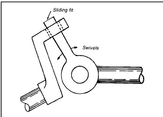
Figure 3-29 This light-duty coupling is ideal for many simple, low-cost mechanisms. The sliding swivel-rod must be kept well lubricated at all times.
