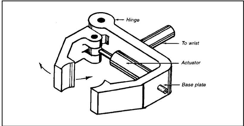
Figure 10-20 Linear actuator direct drive gripper
