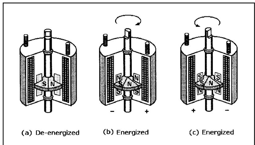
**Figure 1-54** This bidirectional rotary actuator has a permanent magnet disk mounted on its armature that interacts with the solenoid poles. When the solenoid is deenergized (a), the armature seeks and holds a neutral position, but when the solenoid is energized, the armature rotates in the direction shown. If the input voltage is reversed, armature rotation is reversed (c).
