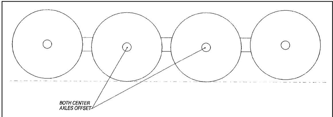
Figure 4-27 Eight wheels, all fixed, center axles offset
