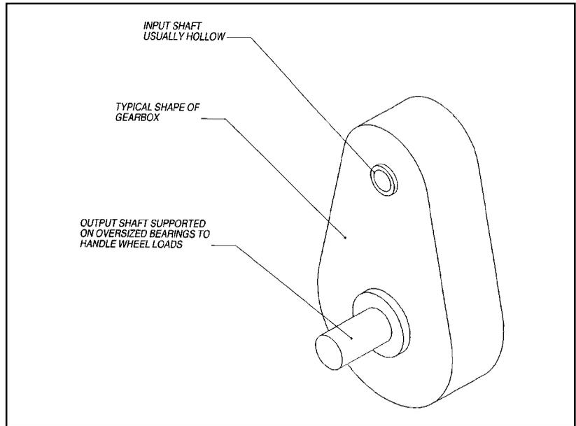
Figure 4-3 Geared offset wheel hub
