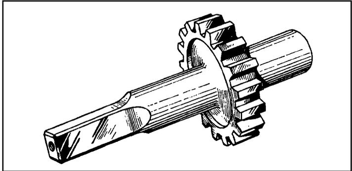
**Figure 3-35** Serrations of small size are used mostly for transmitting light loads. This shaft forced into a hole of softer material makes an inexpensive connection. Originally straight-sided and limited to small pitches, 45° serrations have been standardized (SAE) with large pitches up to 10 in. dia. For tight fits, the serrations are tapered.
