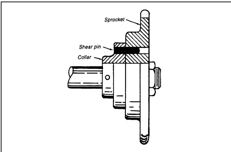
**Figure 3-54** A shear pin is a simple and reliable torque limiter. However, after an overload, removing the sheared pin stubs and replacing them with a new pin can be time consuming. Be sure that spare shear pins are available in a convenient location.
