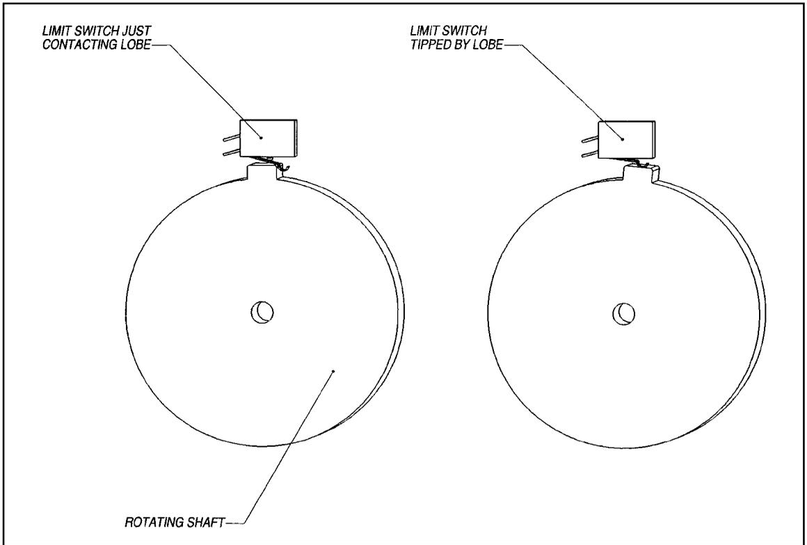
**Figure 11-10** Rotating cam
