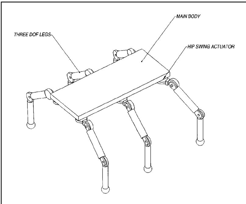
Figure 7-9 Independent leg walker, six legs, eighteen DOF
