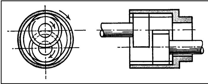
**Figure 3-30** One method of coupling shafts makes use of gears that can replace chains, pulleys, and friction drives. Its major limitation is the need for adequate center distance. However, an idler can be used for close centers, as shown. This can be a plain pinion or an internal gear. Transmission is at a constant velocity and there is axial freedom.
