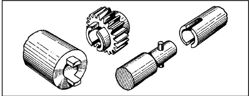
**Figure 3-42** Radical Serrations made by milling or shaping the teeth form simple connections. (A) Tooth proportions decrease radially. (B) Teeth can be straight-sided (castellated) or inclined; a 90° angle is common.
