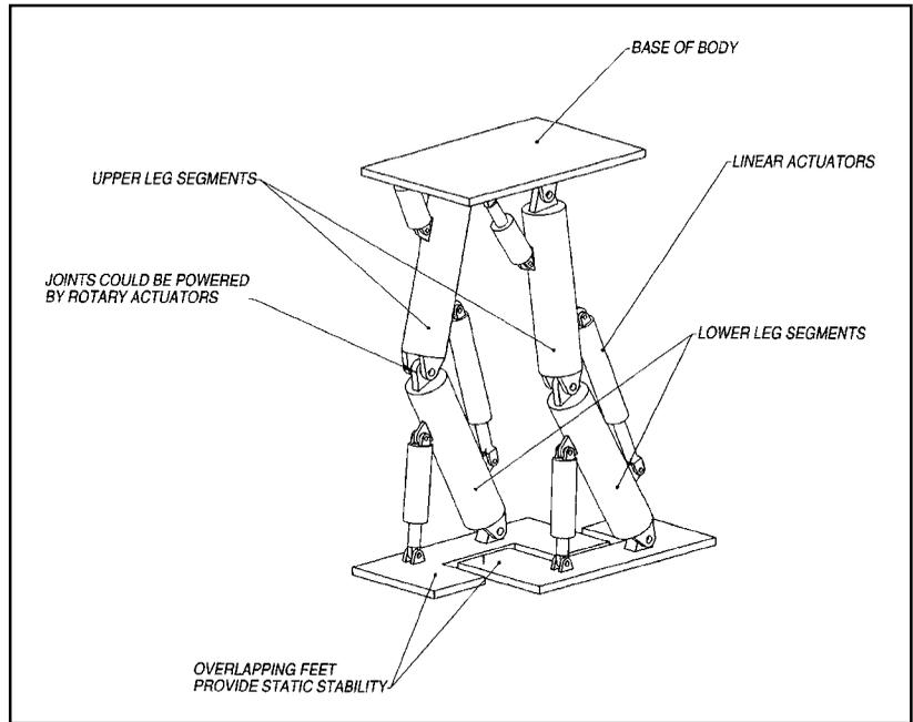
**Figure 7-10** Extra wide feet provide two-legged stability
