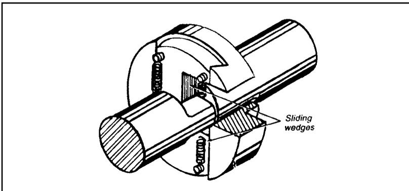
**Figure 3-50** Sliding wedges clamp down on the flattened end of the shaft. They spread apart when torque becomes excessive. The strength of the springs in tension that hold the wedges together sets the torque limit.
