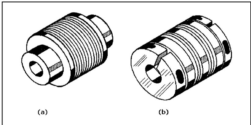
**Figure 1-16** Bellows couplings (a) are acceptable for light-duty applications. Misalignments can be 9° angular or 1/4 in. parallel. Helical couplings (b) prevent backlash and can operate at constant velocity with misalignment and be run at high speed.
