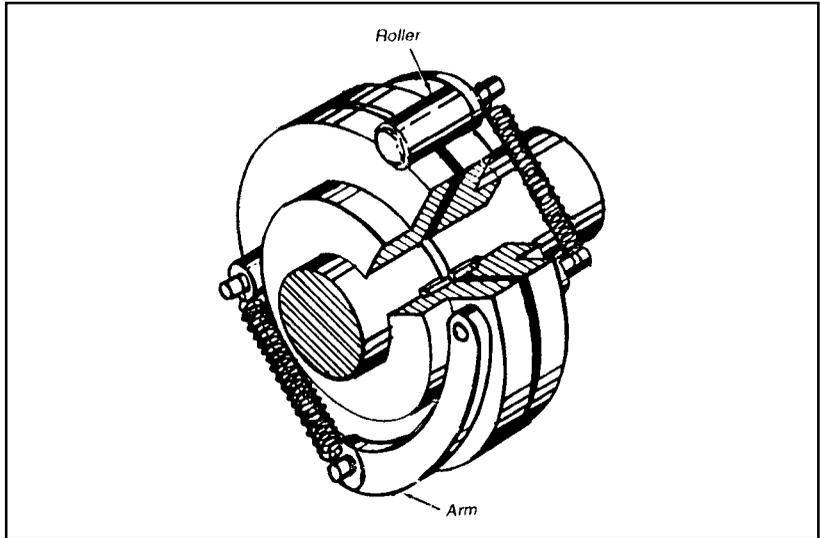
**Figure 3-46** A cone clutch is formed by mating a taper on the shaft to a beveled central hole in the gear. Increasing compression on the spring by tightening the nut increases the drive's torque capacity.
