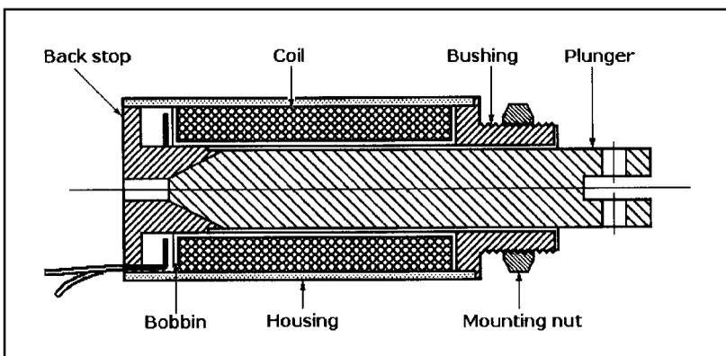
**Figure 1-51** Cross-section view of a commercial linear pull-type solenoid with a clevis. The conical end of the plunger increases its efficiency. The solenoid is mounted with its threaded bushing and nut.
