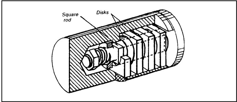
**Figure 3-52** Friction clutch torque limiter. Adjustable spring tension holds the two friction surfaces together to set the overload limit. As soon as an overload is removed, the clutch reengages. A drawback to this design is that a slipping clutch can destroy itself if it goes undetected.
