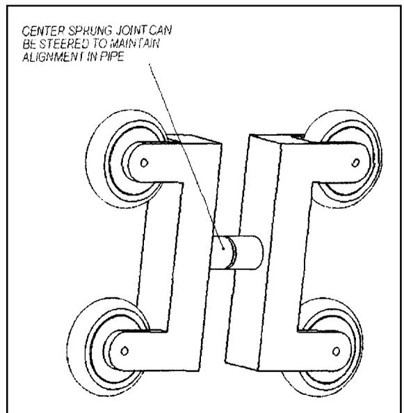
Figure 8-4 Four-wheeled, center steer
