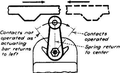
Machine operated lever to provide staggered operating sequence
