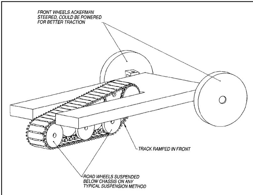
Figure 5-12 One track, two front wheels, Ackerman steer
