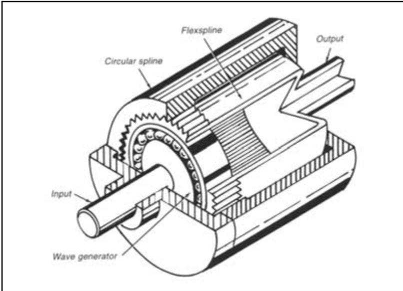
**Figure 2-22** Exploded view of a typical harmonic drive showing its principal parts. The flexspline has a smaller outside diameter than the inside diameter of the circular spline, so the elliptical wave generator distorts the flexspline so that its teeth, 180° apart, mesh.
