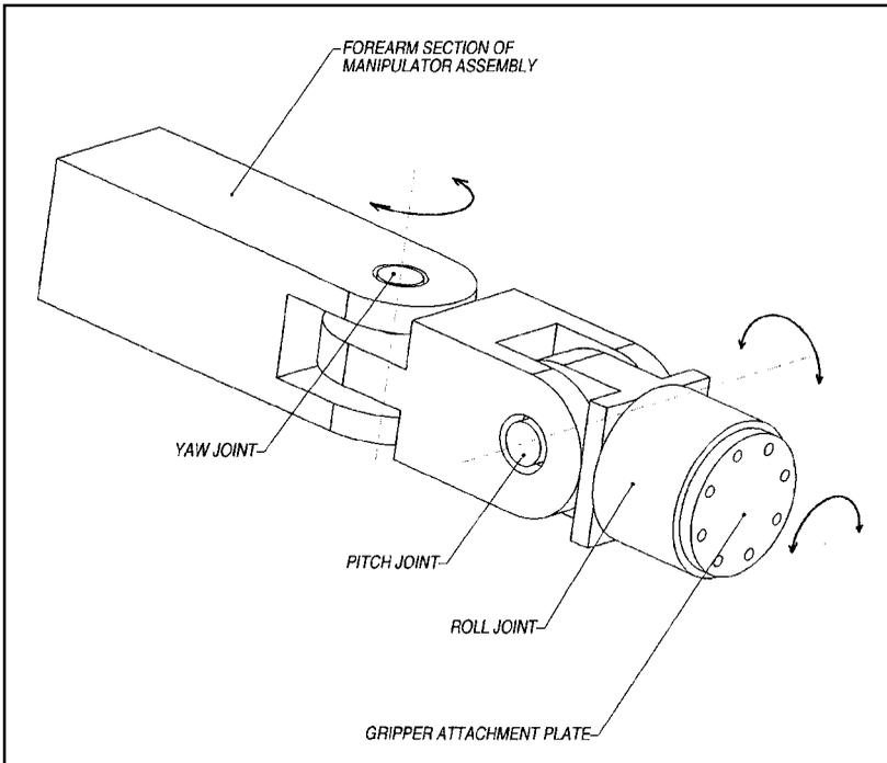
Figure 10-15 Three-DOF wrist (yaw, roll, and pitch)
