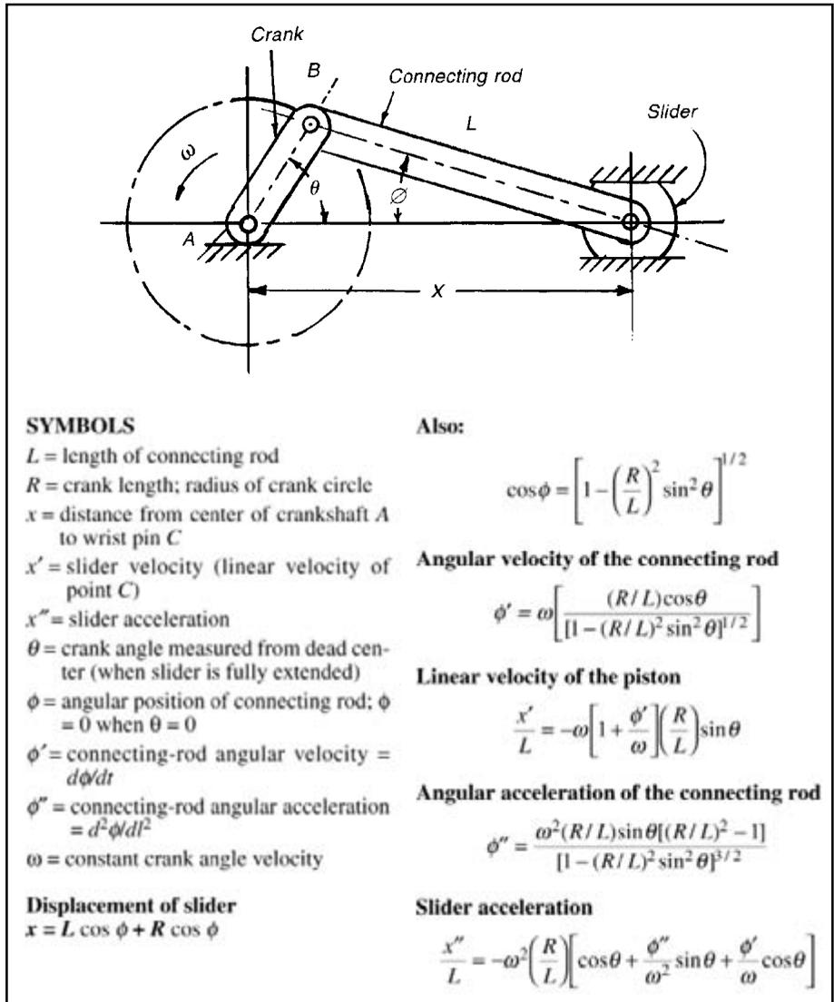
Figure 10-2 Slider Crank
