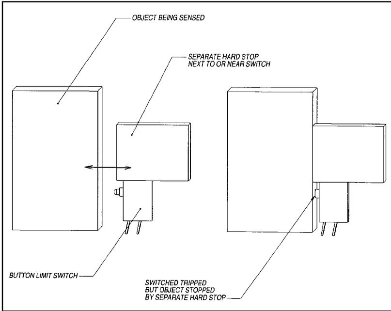
**Figure 11-8** Direct sensing with separate hard stop
