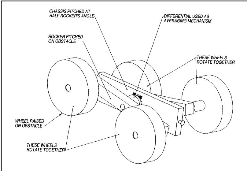
**Figure 4-16** Chassis pitch averaging mechanism using differential
