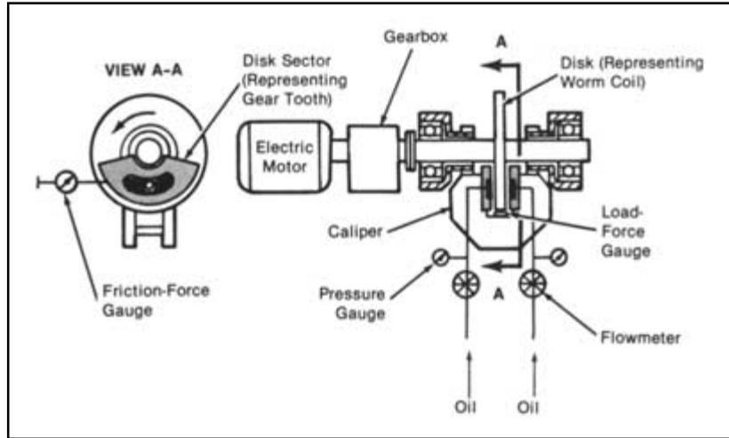
**Figure 2-17** This test apparatus simulates and measures some of the loading conditions of the proposed worm gear with hydrostatic engagement. The test data will be used to design efficient worm-gear transmissions.
