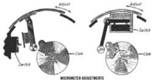
Figure 11-6 Limit Switches in Machinery
