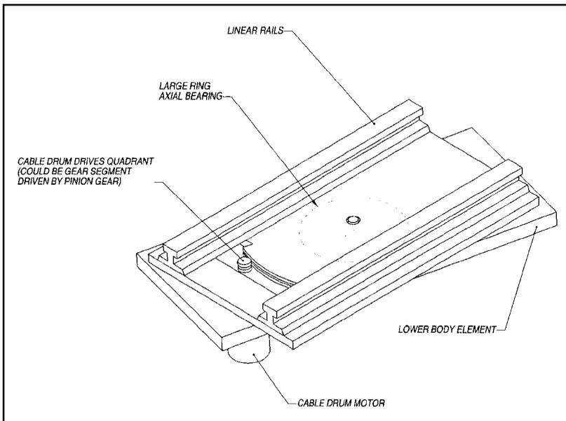
Figure 7-11 Mechanism for frame traversing and rotating
