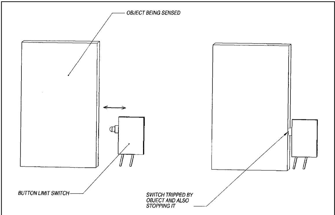
Figure11-7 Direct sensing combined with direct hard stop
