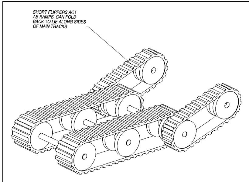
**Figure 5-16** iRobot's Urbie, a four-tracked teleoperated robot layout
