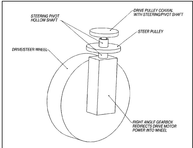
Figure 6-7 Synchronous drive
