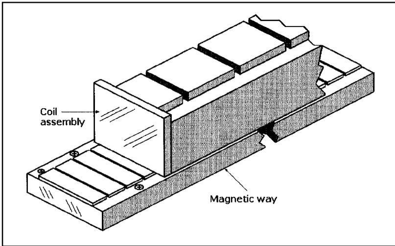
**Figure 1-28** A linear iron-core linear servomotor consists of a magnetic way and a mating coil assembly.
