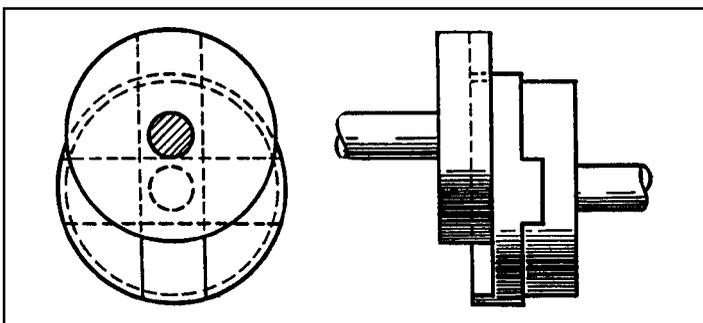
**Figure 3-33** This Oldham coupling provides motion at a constant velocity as its central member describes a circle. The shaft offset can vary, but the shafts must remain parallel. A small amount of axial freedom is possible. A tilt in the central member can occur because of the offset of the slots. This can be eliminated by enlarging its diameter and milling the slots in the same transverse plane.
