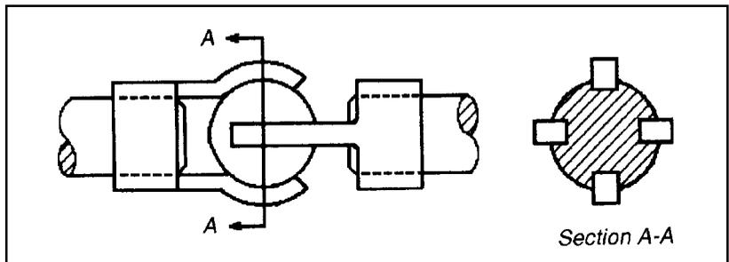
**Figure 3-22** A grooved-sphere joint is a modification of a pinned sphere. Torques on fastening sleeves are bent over the sphere on the assembly. Greater sliding contact of the torques in grooves makes simple lubrication essential at high torques and alignment angles.
