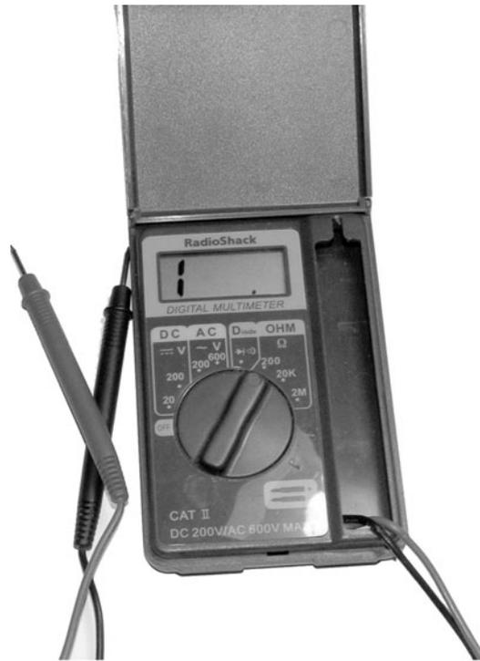
Fig. 5-23. Multimeter.
