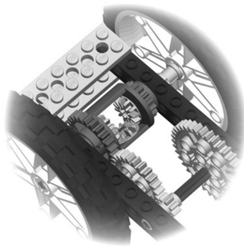
Fig. 9-26. Differential power transmission.
