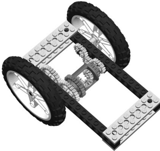
Fig. 9-27. Differential to measure turn angle.
