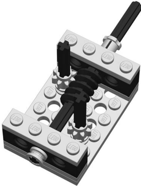
Fig. 9-24. Worm gear reverser.
