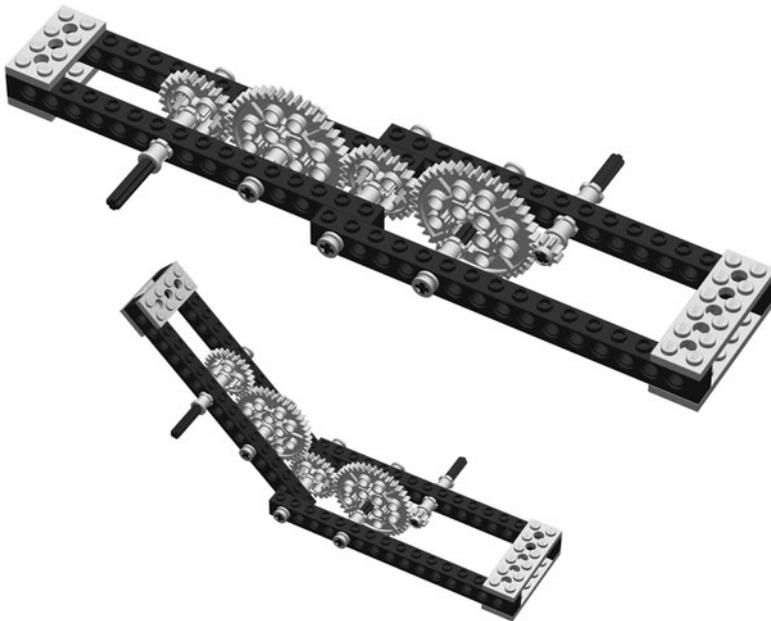
Fig. 9-14. Gears around a corner.
