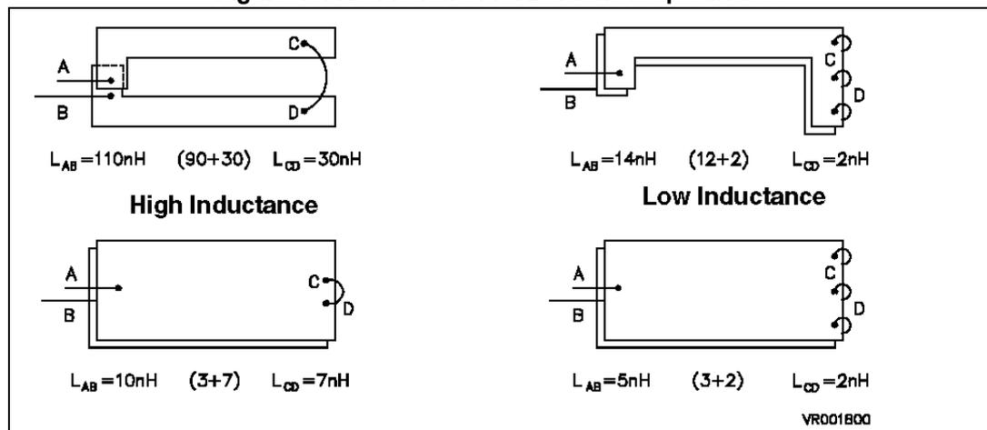
Note: This test is done with a double sided PCB. Insulator thickness is 1.5 mm, copper thickness is 0.13 mm. The overall board size is 65 x 200 mm.
