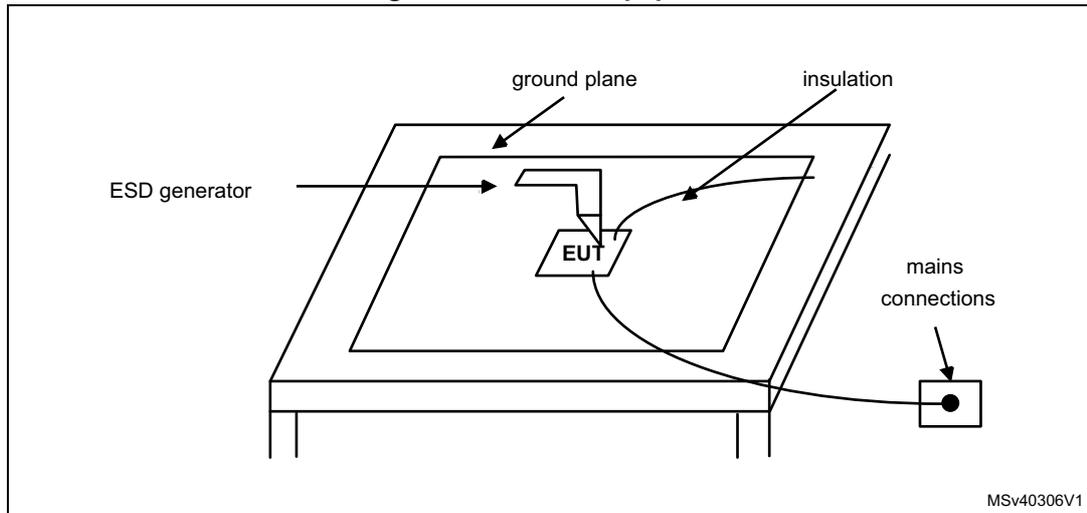
The equipment used to perform F\_ESD test is a NSG 435 generator (TESEQ) compliant with the IEC 61000-4-2 standard. The discharges are directly applied on each pin of the MCU.
