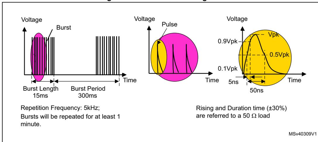
The spike frequency is 5 kHz. The generator produces bursts of spikes that last 15 ms every 300 ms (75 spikes).
