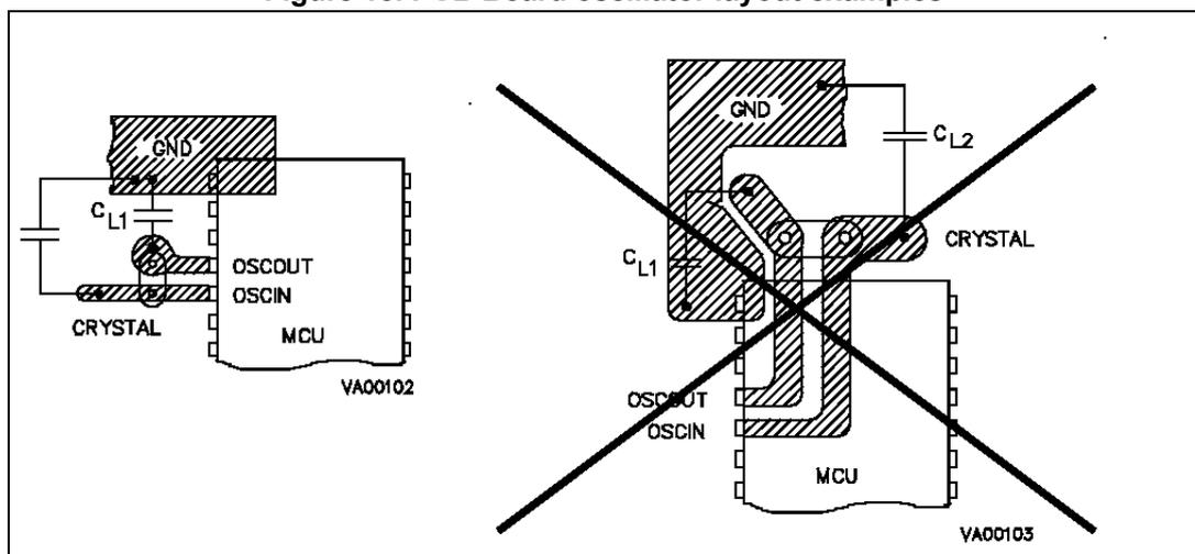
The reduction of inductance can be obtained by making the lengths and surfaces of the track smaller. This can be obtained by placing the track loops closer on the same PCB layer or on top of one another (Figure 19). The resulting loop area is small and the electromagnetic fields reduce one another.
