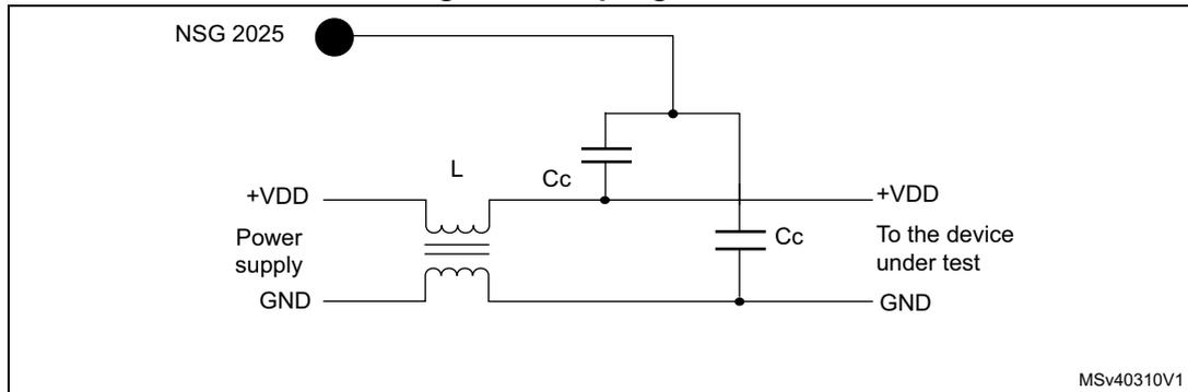
Measurements are performed on a ground plane. The generator is connected to ground plane by a short wire. The supply wires are 10 cm from the ground plane. The DUT is on the insulator 10 cm from the ground plane. The FTB voltage level is increased until the device failure.
