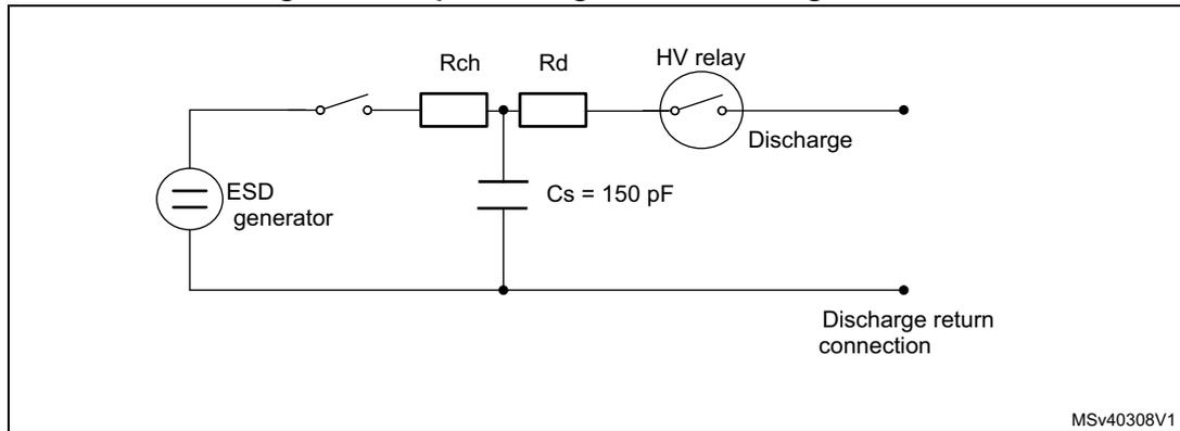
1.  $R_{ch} = 50 \text{ M}\Omega$  ;  $R_d = 330 \text{ }\Omega$  .
