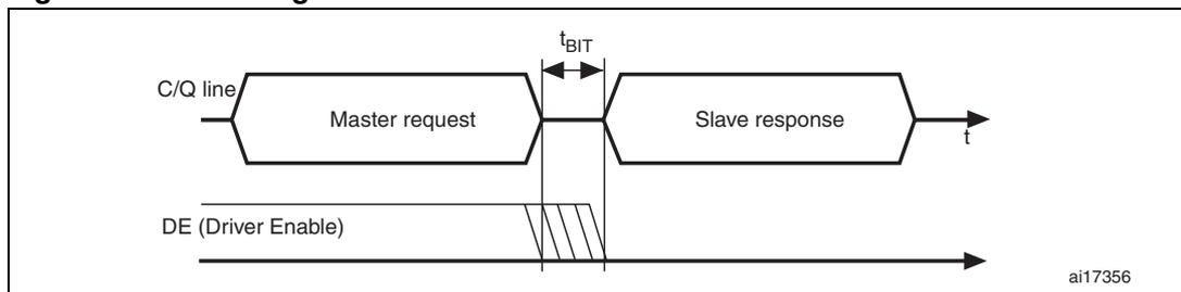
The master should be able to guarantee the timing of the DE signal (imposed by the RS-485 & IO-Link specifications). The DE signal is managed by a GPIO.
