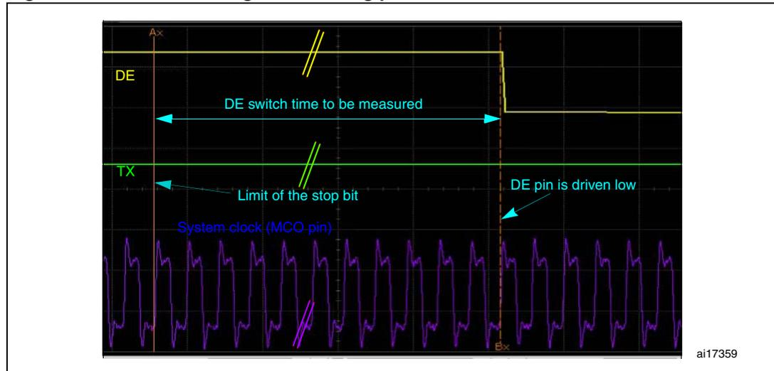
The MCO pin (PA8) is used to output the system clock (CPU clock) in order to measure in CPU cycles the time taken by the DE signal to switch to the low level.
