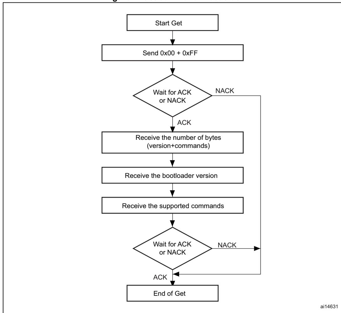
Figure 3. Get command: device side
