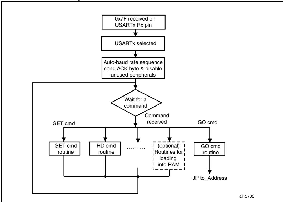
Once the system memory boot mode is entered and the STM32 microcontroller has been configured (for more details refer to application note AN2606 “STM32 system memory boot mode”) the bootloader code begins to scan the USARTx\_RX line pin, waiting to receive the 0x7F data frame: one start bit, 0x7F data bits, even parity bit and one stop bit.
