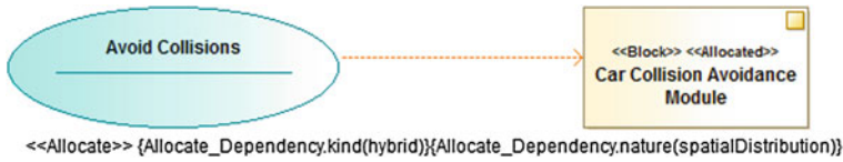
Fig. 10 Mapping the Avoid Collisions use case to the Car Collision Avoidance Module block
