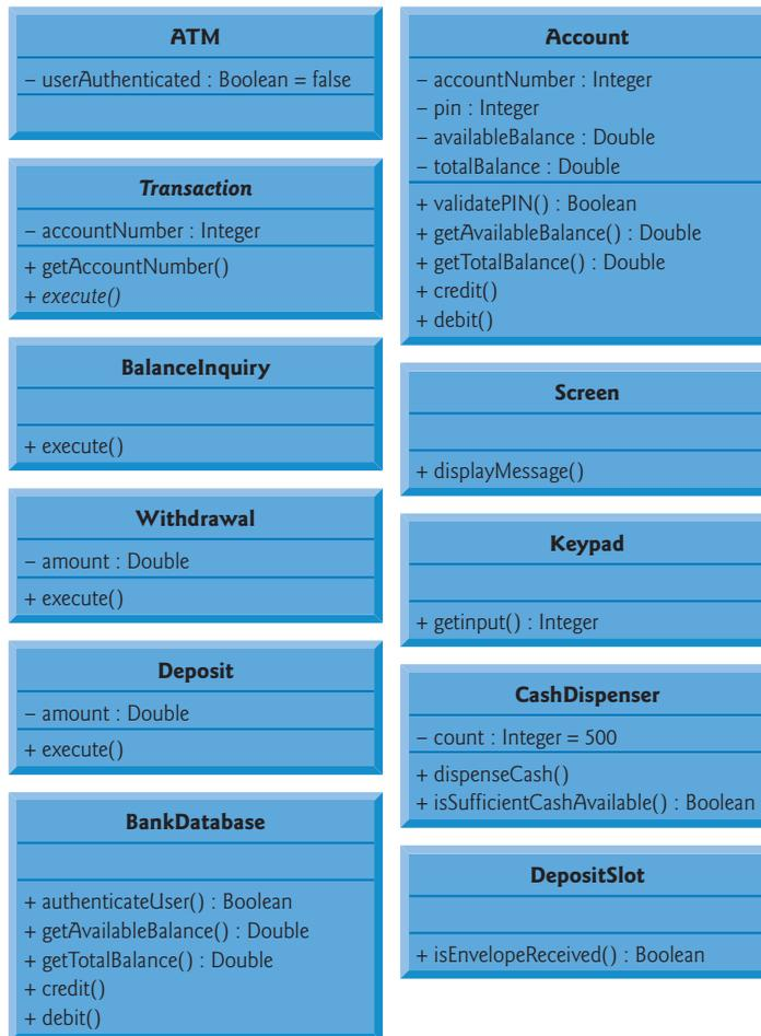
**Fig. 26.11** | Class diagram after incorporating inheritance into the system.
