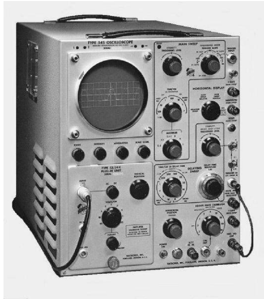
Figure 1-28: Tektronix introduced the 545 scope back in the dark ages; A half-century later many are still going strong. Replace a tube from time to time and these might last forever. About the size of a two drawer file cabinet and weighing almost 100 pounds, they're still favored by Luddites and analog designers.
