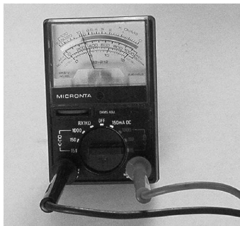
Figure 1-2: A VOM, even an old-fashioned analog model like this $10 Radio Shack model, measures DC voltage as well or better than a scope.
