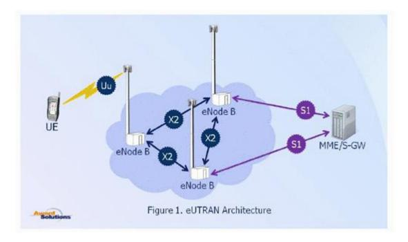
Figure 1 illustrates an LTE eUTRAN, the radio access network. The eUTRAN has a flat architecture with no centralized controller; instead each eNodeB manages its own radio resources and collaborates with other eNodeB's over the X2 interface. The eNodeB's connect to the core network over the S1 interface to allow users to register with the network and send and receive traffic.
