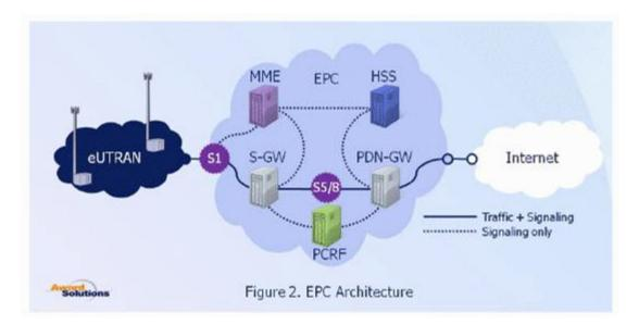
Key LTE terms associated with the core network, and their 1xEV-DO equivalents, are listed here:
