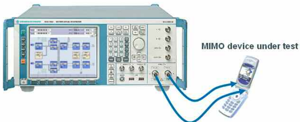
Figure 36 Downlink MIMO receiver test: Signal generator SMU200A provides LTE downlink signals from two transmit antennas including channel simulation
