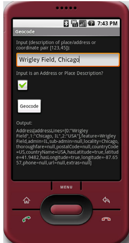
Figure 11.8 A Geocoder usage example that demonstrates turning an Address String into an Address object that provides latitude and longitude coordinates
