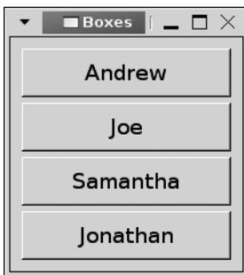
**Figure 3-1.** A vertical box packed from the start position
