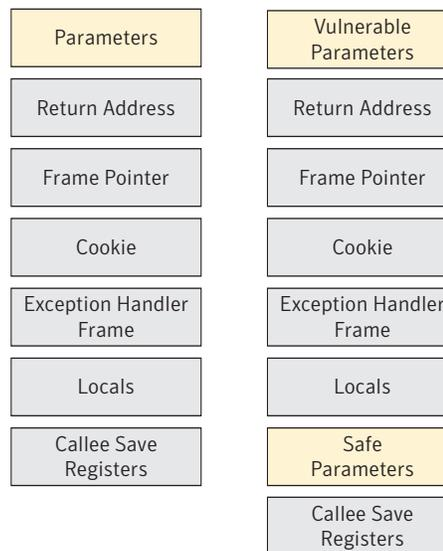
**Figure 2. Stack frame layouts used in Visual Studio 2003 (left) and 2005 (right)**
