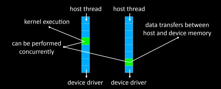
Overlap of data transfer and kernel execution transfer data between host page-locked memory and device memory and kernel execution can be performed concurrently any application may query the hardware capability by calling
