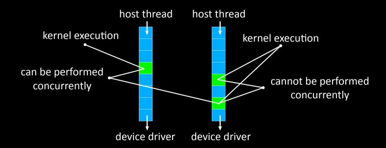
Concurrent kernel execution some hardware can execute multiple kernels concurrently any application may query the hardware capability by calling the device manage function and checking the property flag
