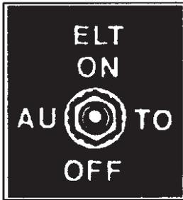
**ON:** used to remotely activate the transmitter for test or emergency situation. An example of such an emergency situation would be forced landing with an impact insufficient to activate the Rolamite "G"-switch.
