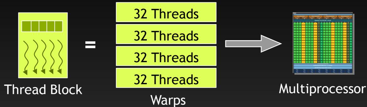
**A thread block consists of 32-thread *warps***
