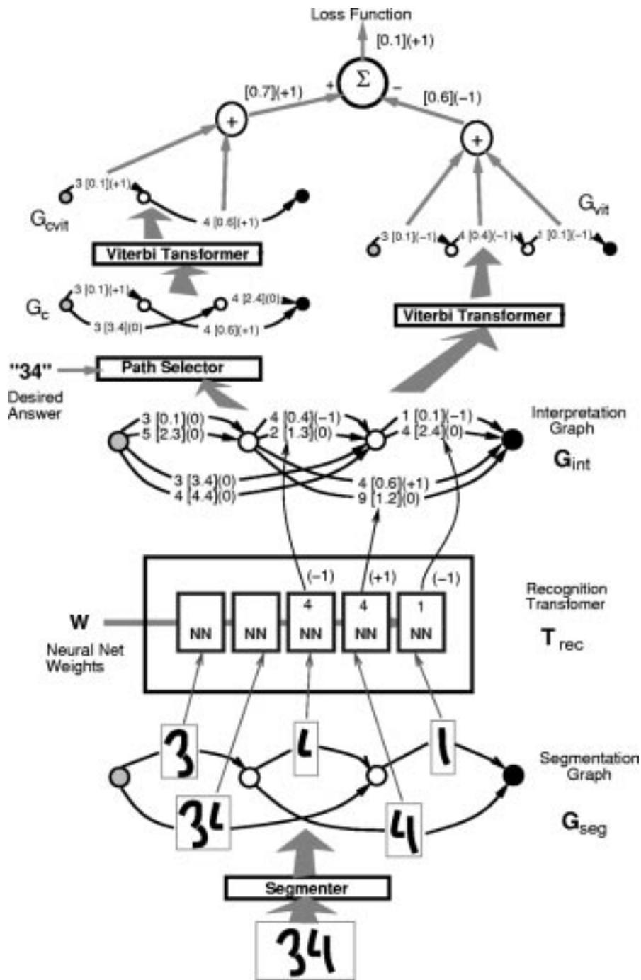
**Fig. 20.** Discriminative Viterbi training GTN architecture for a character string recognizer based on HOS. Quantities in square brackets are penalties computed during the forward propagation. Quantities in parentheses are partial derivatives computed during the backward propagation.
