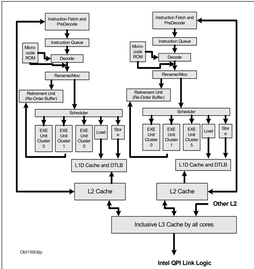
**Figure 2-12. Intel Microarchitecture Code Name Nehalem Pipeline Functionality**
