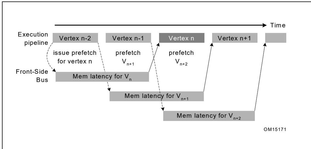
**Figure 7-4. Memory Access Latency and Execution With Prefetch**
