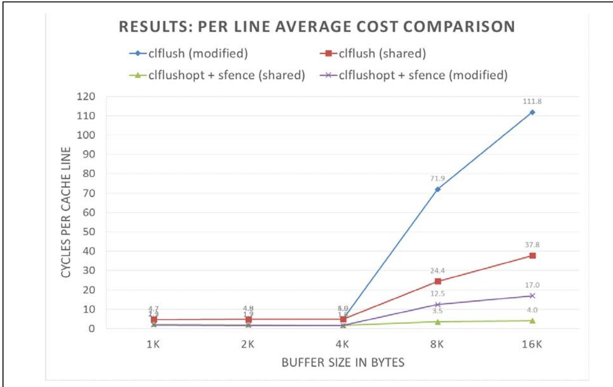
**Figure 7-1. CLFLUSHOPT versus CLFLUSH In SkyLake Microarchitecture**
