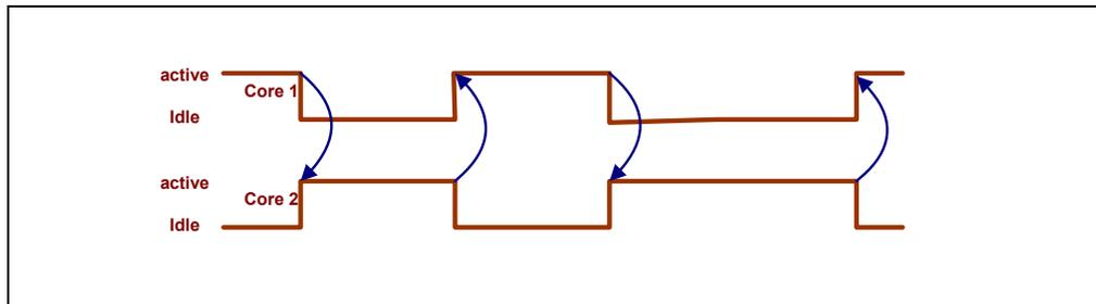
**Figure 14-5. Thread Migration in a Multicore Processor**
