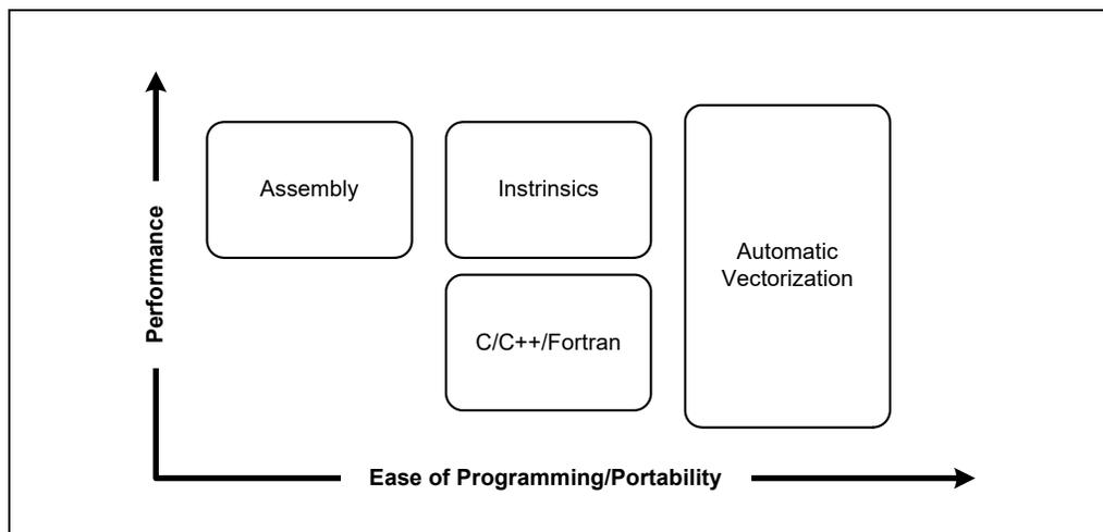
**Figure 4-4. Hand-Coded Assembly and High-Level Compiler Performance Trade-offs**
