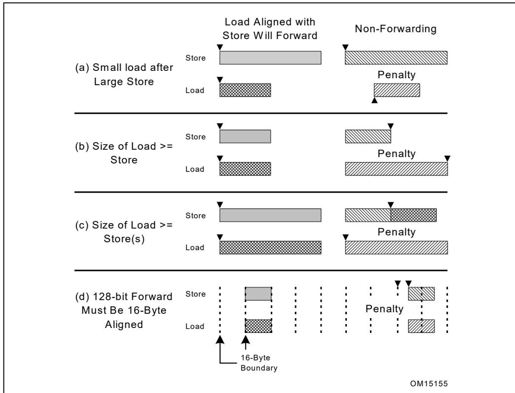
**Figure 3-3. Size and Alignment Restrictions in Store Forwarding**
