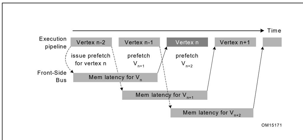
Figure 7-6. Memory Access Latency and Execution With Prefetch
