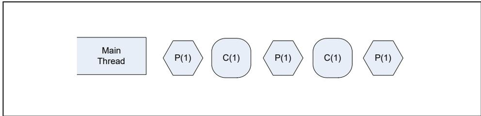
**Figure 9-2. Single-threaded Execution of Producer-consumer Threading Model**
