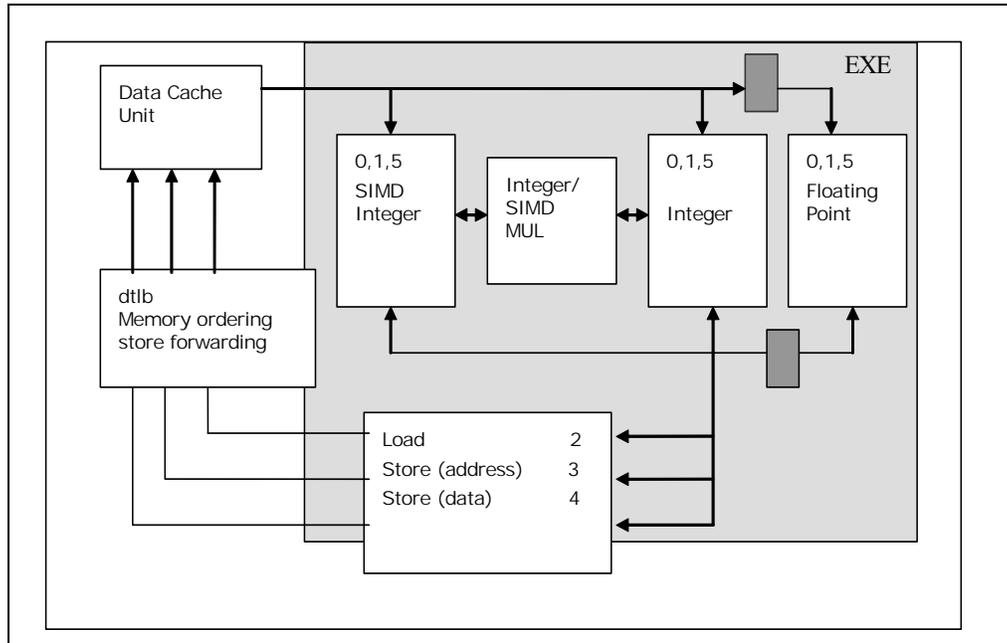
**Figure 2-9. Execution Core of Intel Core Microarchitecture**
