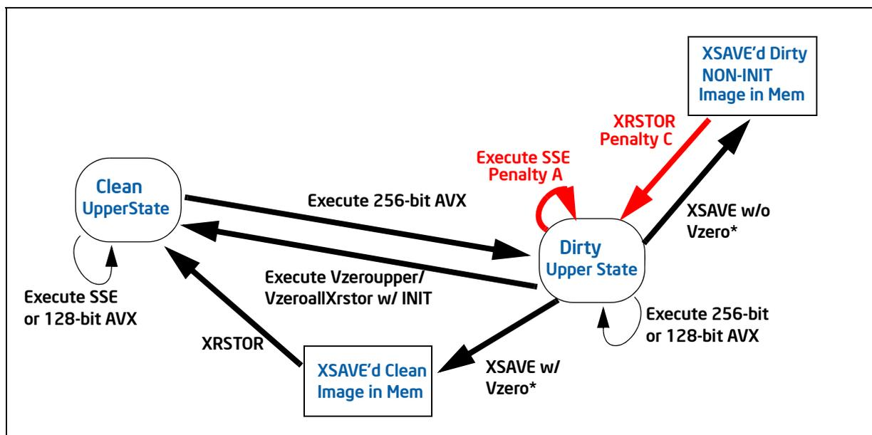
Figure 12-2. AVX-SSE Transitions in the Skylake Microarchitecture
