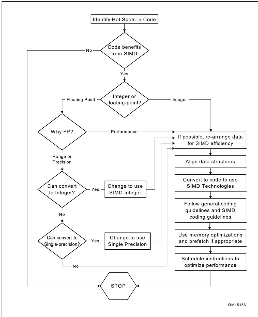
**Figure 4-3. Converting to Streaming SIMD Extensions Chart**
