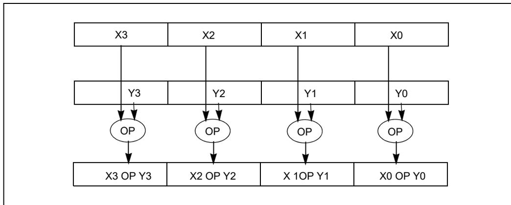
**Figure 6-1. Homogeneous Operation on Parallel Data Elements**
