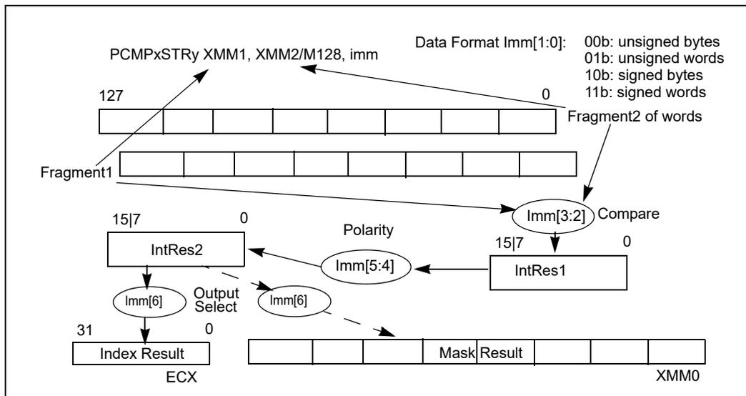
Figure 11-1. SSE4.2 String/Text Instruction Immediate Operand Control
