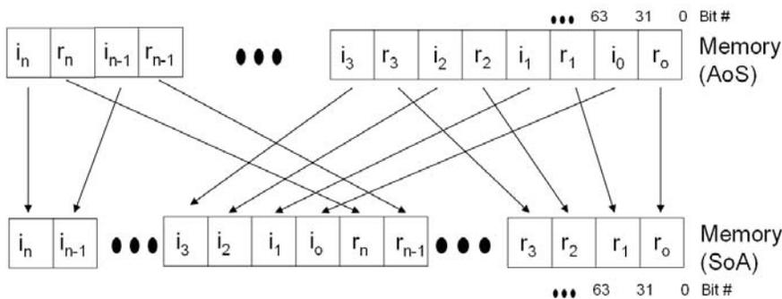
A simple extension of the Intel SSE algorithm from 16-byte to 32-byte operations would require cross-lane data transition, as shown in the following figure. However, this is not possible with Intel AVX architecture and a different technique is required.
