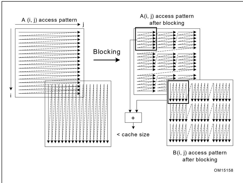
Figure 4-5. Loop Blocking Access Pattern
