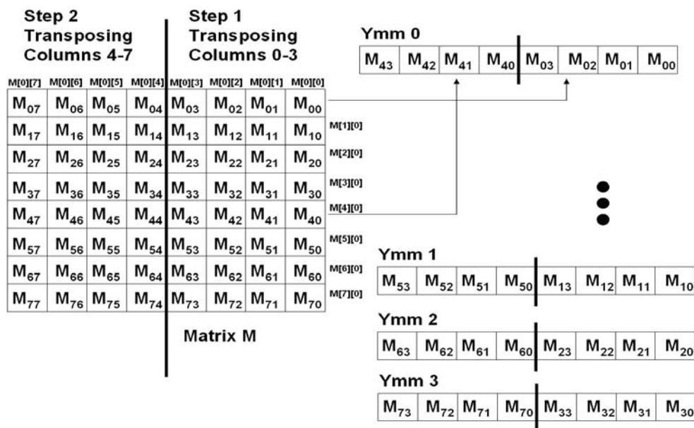
The following figure describes step 1 of the 8x8 matrix transpose with vinsertf128. Step 2 performs the same operations on different columns.
