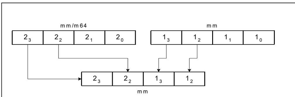
**Figure 5-4. Result of Non-Interleaved Unpack High in MM1**
