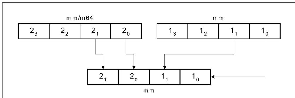
**Figure 5-3. Result of Non-Interleaved Unpack Low in MM0**
