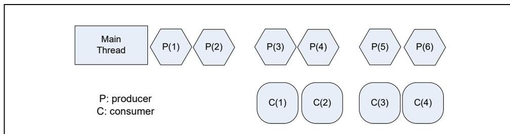
Figure 9-5. Batched Approach of Producer Consumer Model
