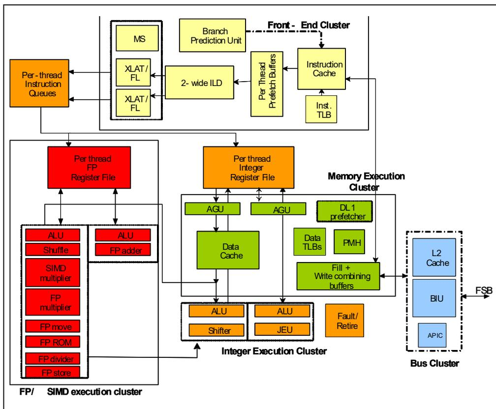
Figure D-1. Intel Atom Microarchitecture Pipeline
