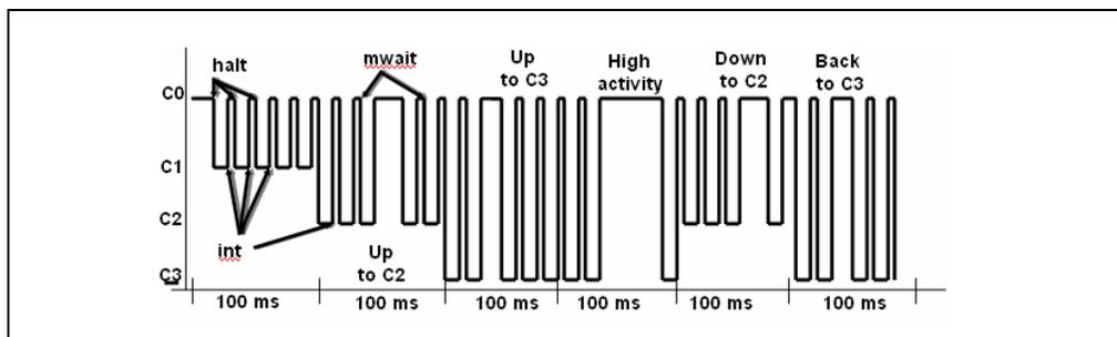
Figure 14-3. Application of C-states to Idle Time
