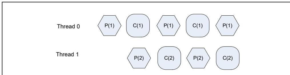
**Figure 9-4. Interlaced Variation of the Producer Consumer Model**
