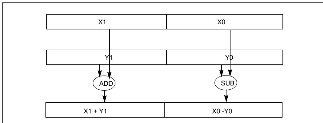
Figure 6-5. Asymmetric Arithmetic Operation of the SSE3 Instruction
