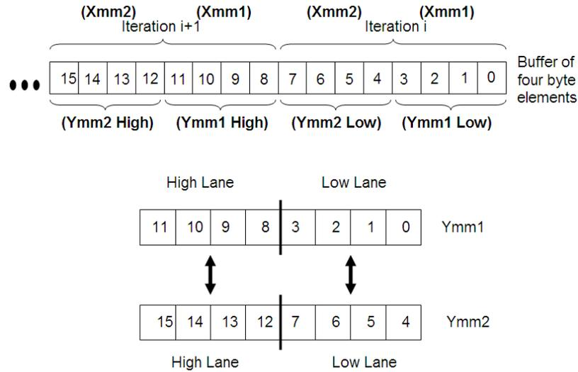
The values in the low lanes of Ymm1 and Ymm2 in the figure above correspond to iteration  $i$  in the SSE implementation. Similarly, the values in the high lanes of Ymm1 and Ymm2 correspond to iteration  $i+1$ .
