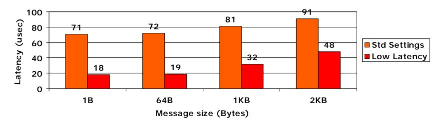
Bensley Platform, Red Hat RHEL4 - Kernel Version 2.6.12.4, Netperf Latency Test - Driver ver. 7.0.16, Driver Parameters Tuned for Low Latency - Interrupt Moderation disabled
