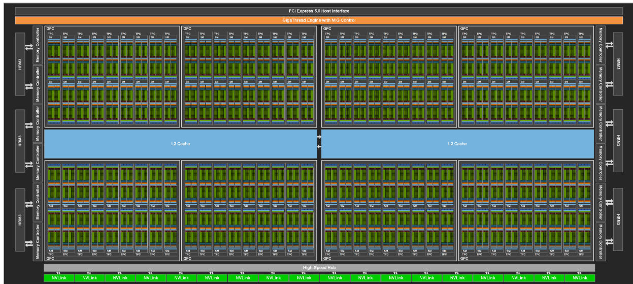
Figure 6. GH100 Full GPU with 144 SMs
