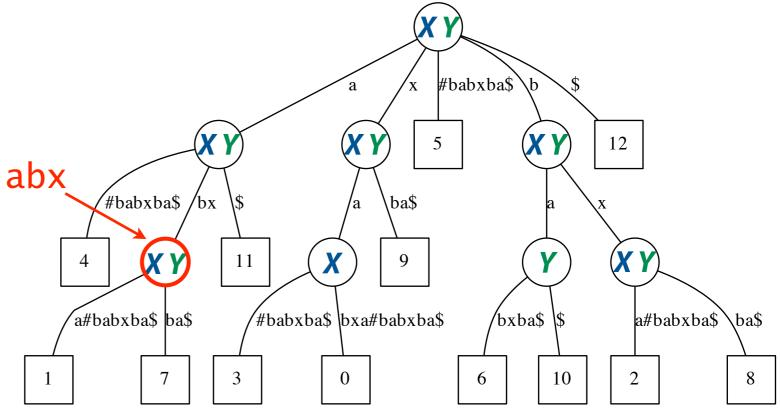
Traverse the tree and annotate each node according to whether leaves below it include suffixes of X, Y or both
