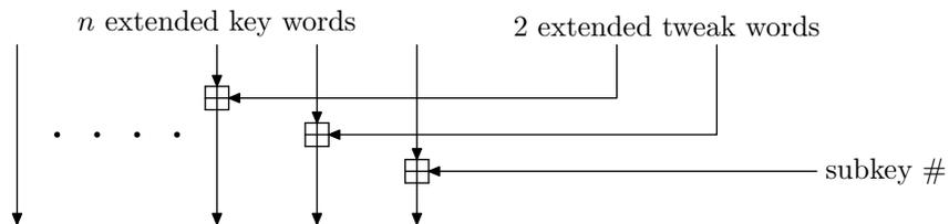
Figure 3: Constructing a Threefish subkey.
